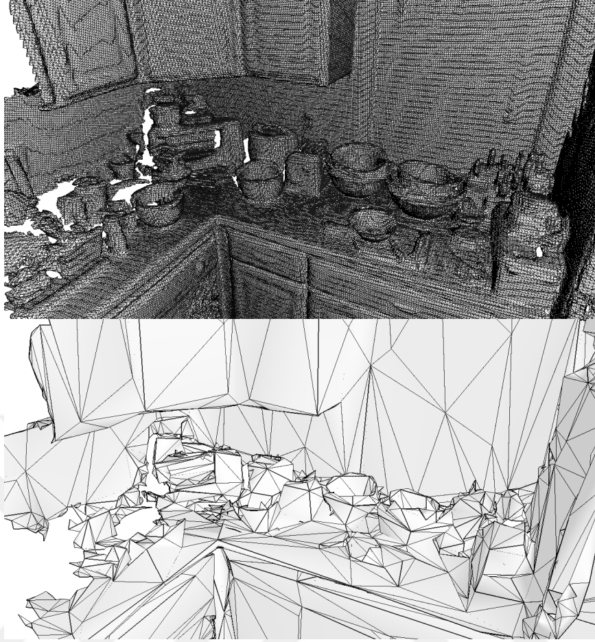
Figure 4.2: Comparison of raw (top) and simplified (bottom) scenes in terms of detail
