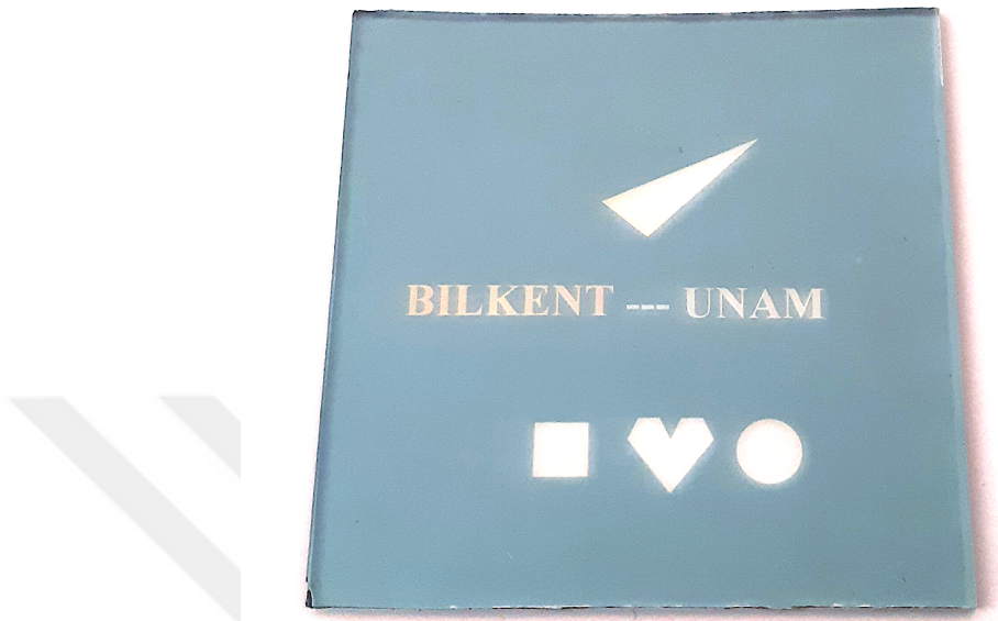
Figure 4.1: Coated glass sample. The writings and the shapes were drawn by ablating the coating with different laser parameters.
