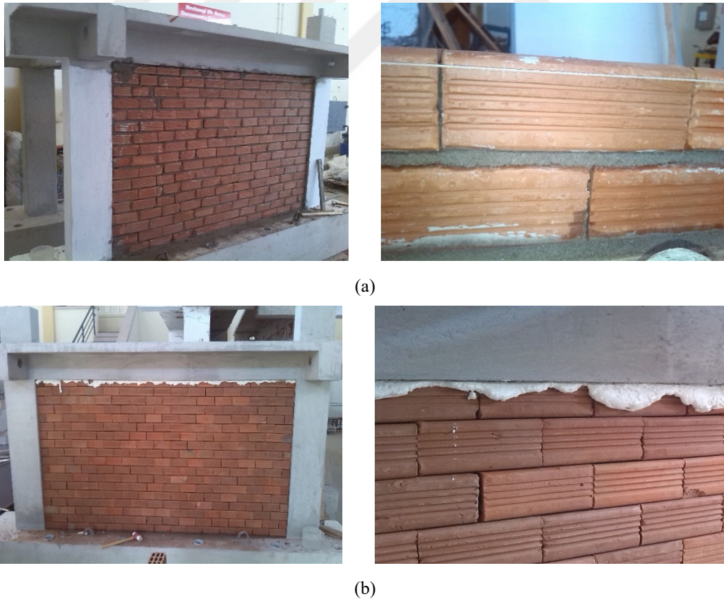
Figure 4.4 General views and interface details for the infill walls constructed with (a) standard and (b) locked type bricks (Personal archive, 2016)
