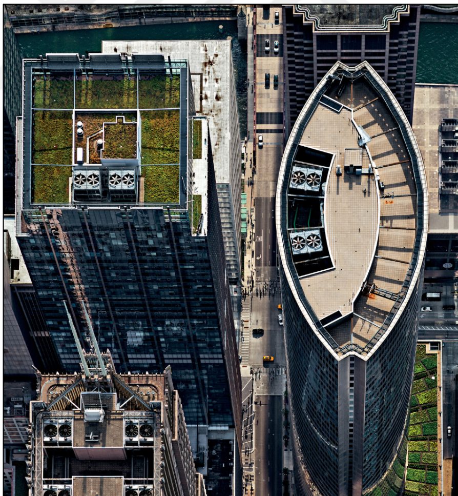
Figure 3.4. Extensive roof sample 111 South Wacker, Chicago [22].
