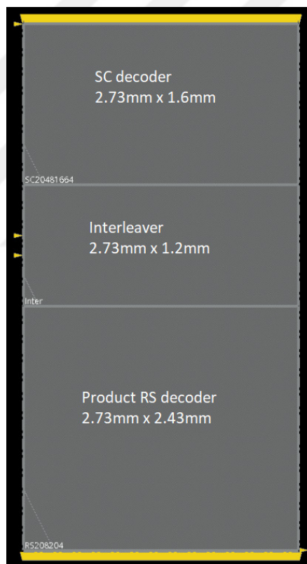
Figure 3.13: Hierarchical floor-planning of RS2-Polar decoder.
