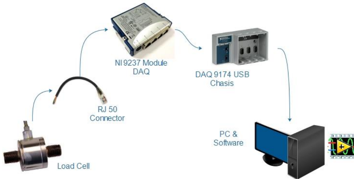
Figure 7.8. Load Cell data acquisition system
