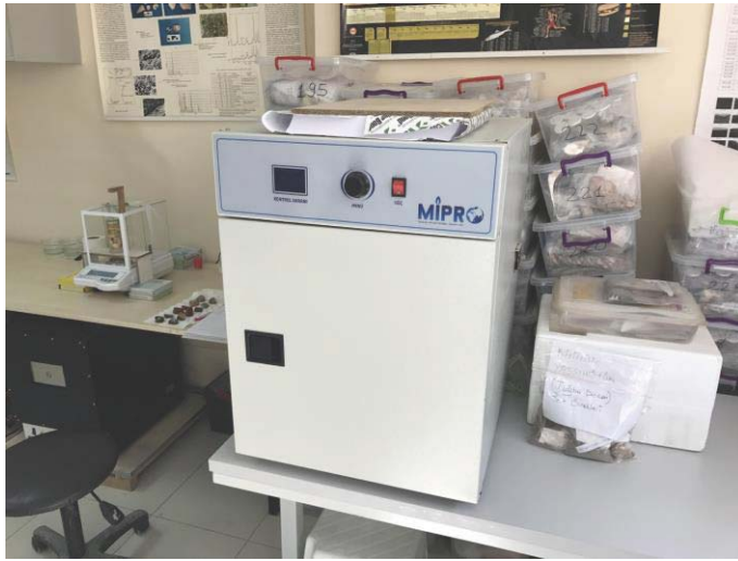
Figure 3.8. Mipro Etiv Dryer used in this study
