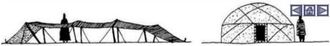
FIG. 2.5. Portable tents of sticks and felt. Left: Arab tent. Right: Mongol Yurt.
