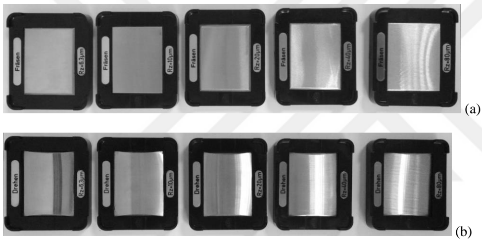
Figure 4.8 Milling (a) and Turning (b) steel samples
