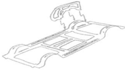
Figure 2.4 The automobile stamped chassis (Anonymous, 2018a)
