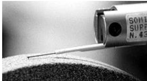
Figure 3.13 Stylus and Pickup working on surface (Anonymous, 2011)
