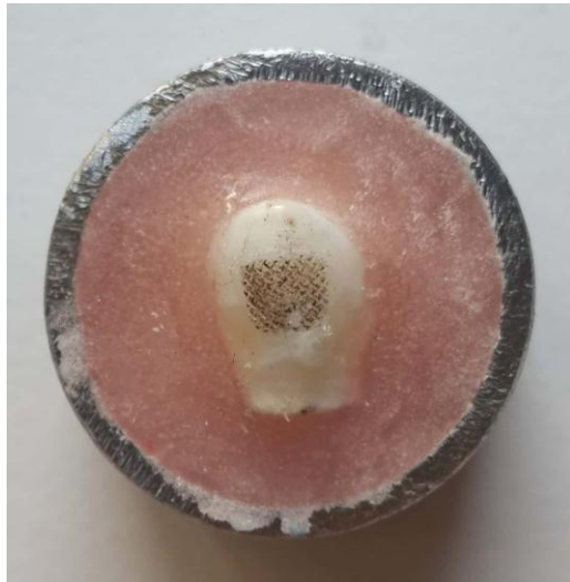
Figure2.31: Distinct impression of the bracket mesh after bracket debonding.
