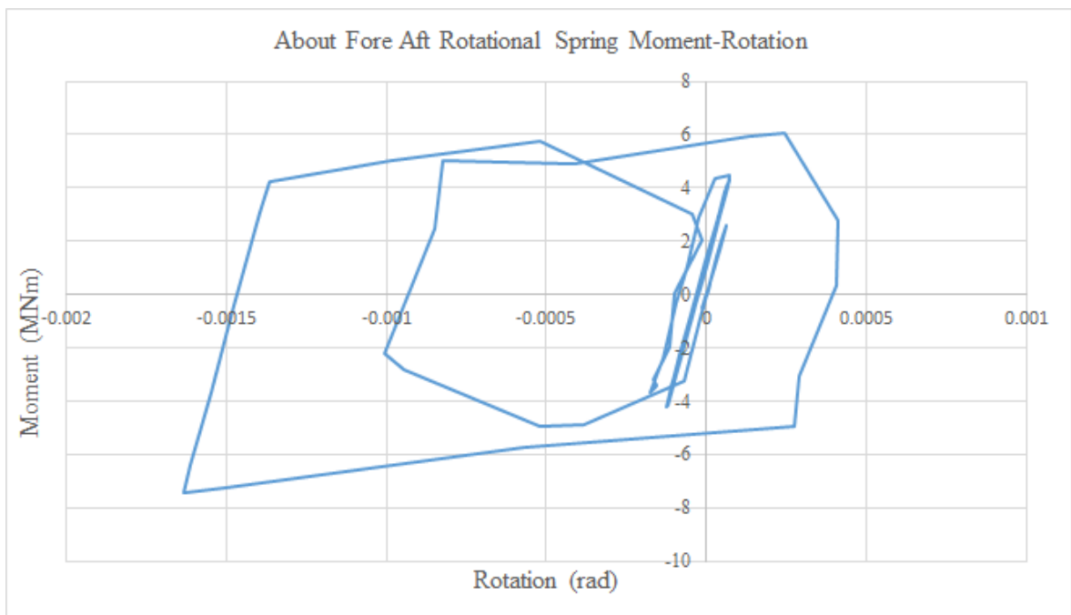
Figure 4.19. Moment vs Rotation about Fore Aft Rotational Spring Under Kocaeli Record.
