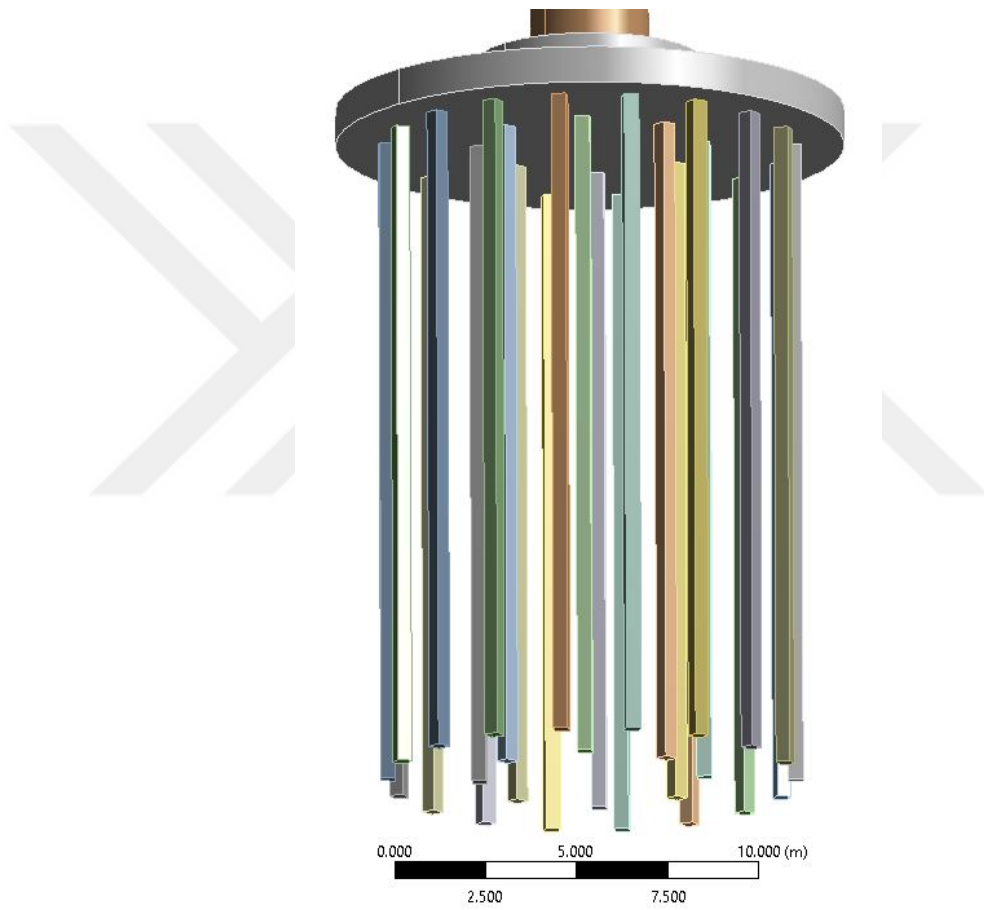
Figure 3.5. Pile Group in the Model.
