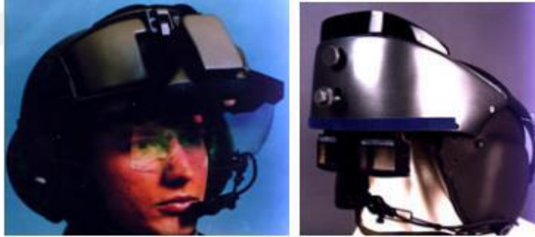
Şekil 4. Başa monte edilen kasklı ekran AG platformu. Azuma, R. T. (1997). A Survey of Augmented Reality. Presence: Teleoperators and Virtual Environments , 6(4), 355-385.
