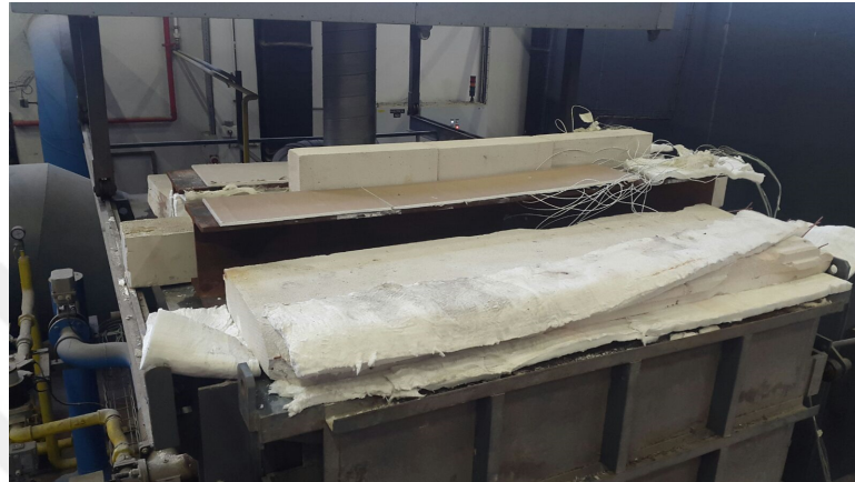
Figure 5.31. General View before the Test for HEB 300.
