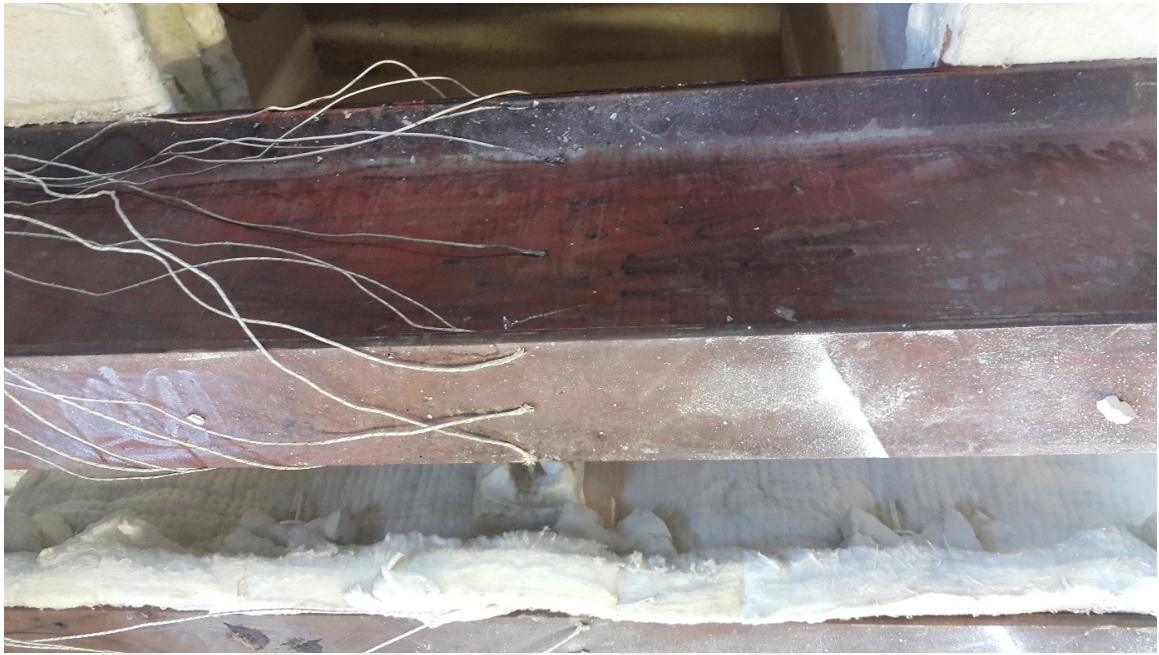
Figure 5.8. Fixed Thermocouples for INP 400.
