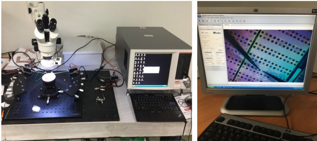
Figure 5.3: I-V measurement platform.
