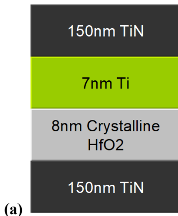
Figure 6.1: 1R part of the 1T1R device having 8 nm crystalline HfO 2 layer as the memory environment.
