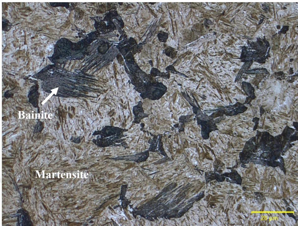
Figure 26. Optical micrograph of R260 steel, quenched to 170°C and hold isothermally for 3 hours.
