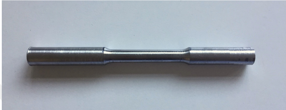
Figure 22. Tension test specimen of 32CrBr steel
