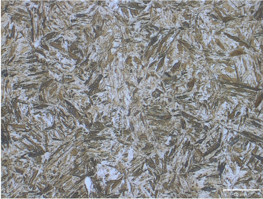
Figure 33. Optical image of fully martensite phase of 32CrB4 steel, obtained by water quenching
