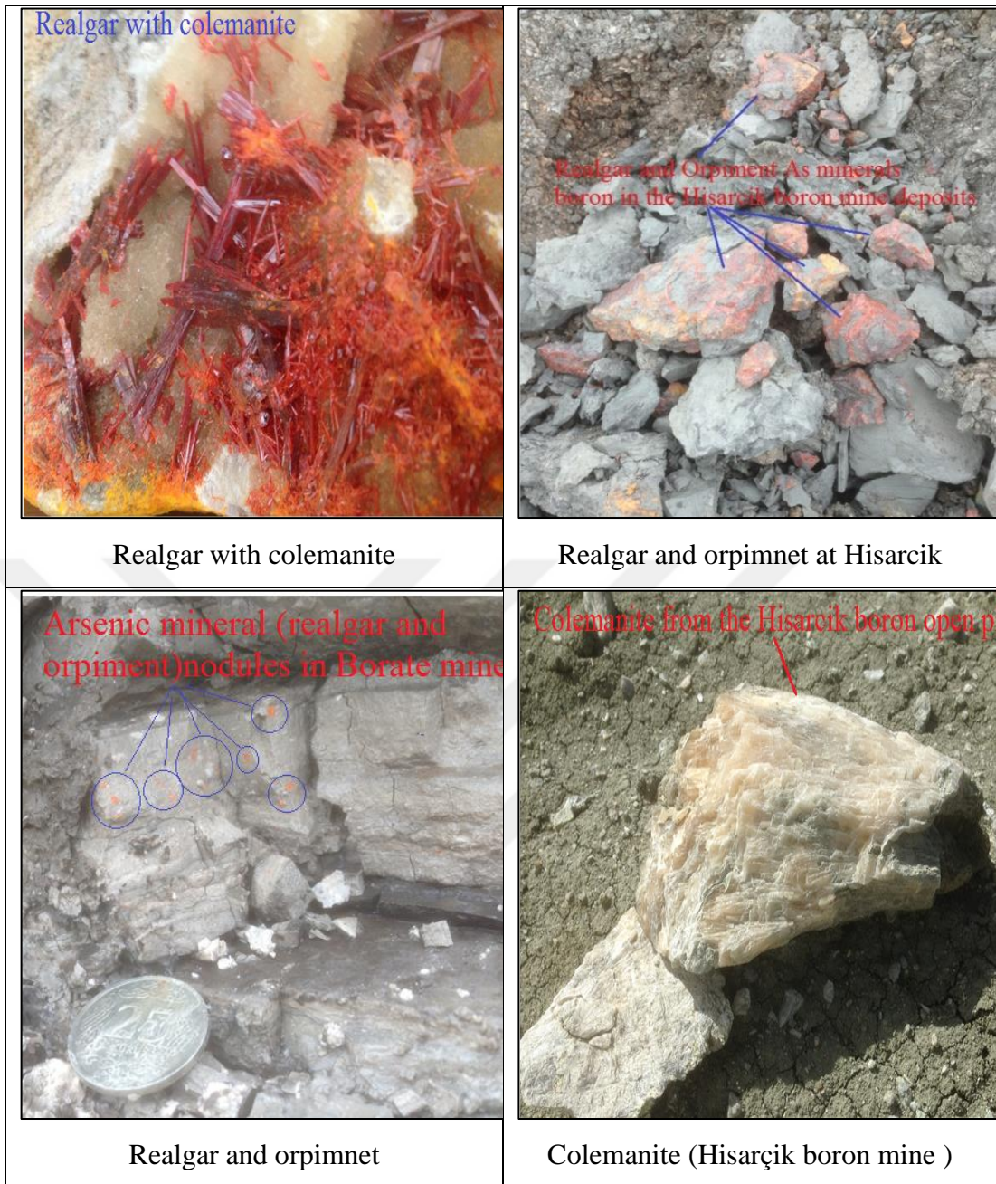
Figure 2.12: Photographs of some arsenic minerals (Realgar, Orpiment and Colemanite) in Emet-Hisarcik Open Pit Boron Mines.
