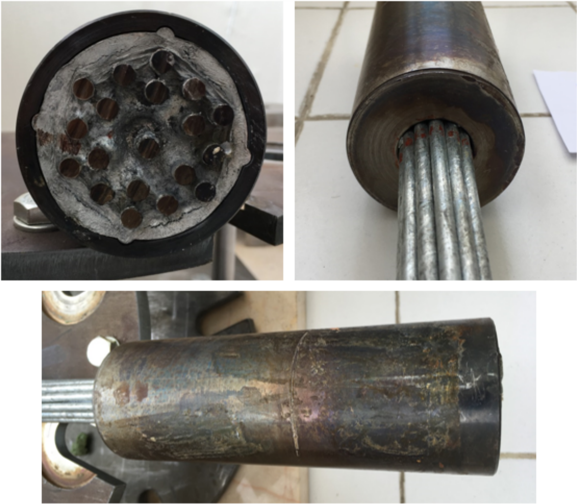
Figure 4.23. Condition of dead end socket after fire test.
