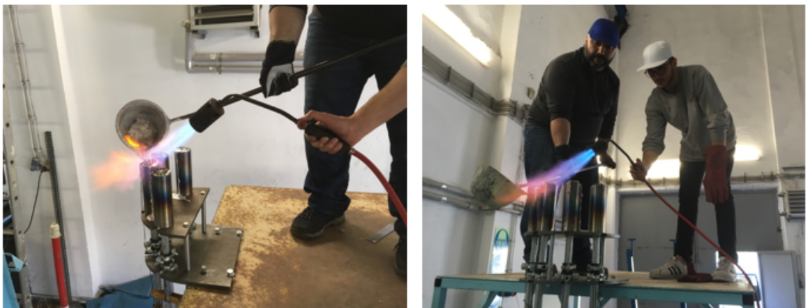
Figure 3.22. Hot casting operation by competent founders.
