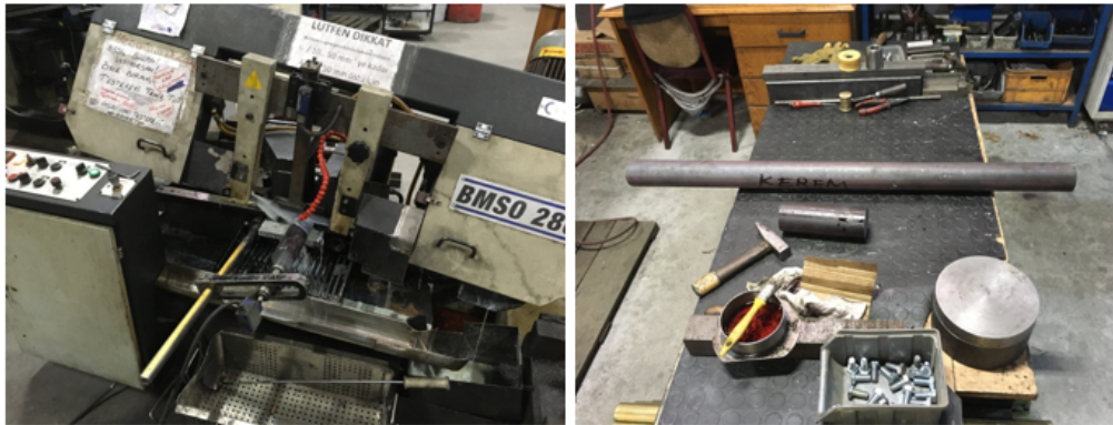
Figure 3.11. Band saw machine (left-hand side), Mild steel bar and cut bar (right-hand side).
