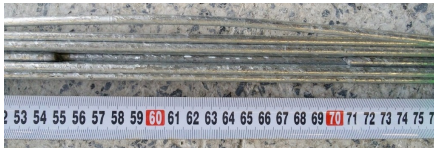
Figure 4.7. The ruptured wire position for S2.
