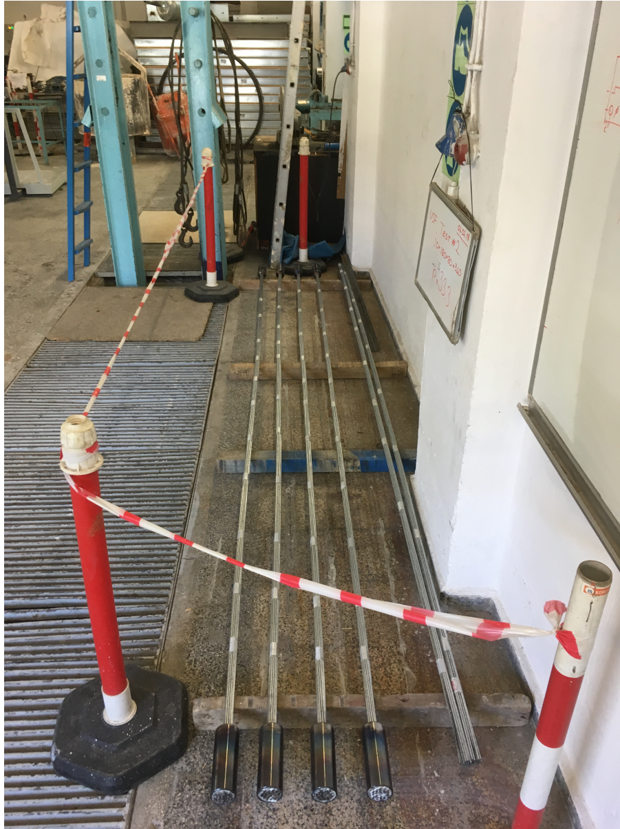
Figure 3.23. Pictures of test specimens assembled by hot casting method.
