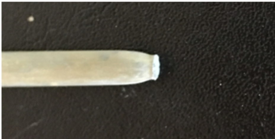
Figure 4.20. A typical cup and cone wire rupture for S3.
