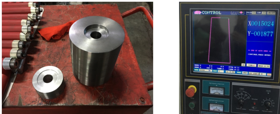
Figure 3.35. View of the socket lockers after machining process and EDM control panel.
