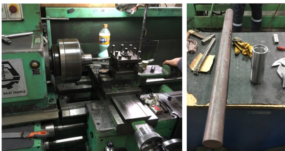
Figure 3.12. Lathe machine mild steel bar (left-hand side) and machined socket material (right-hand side).
