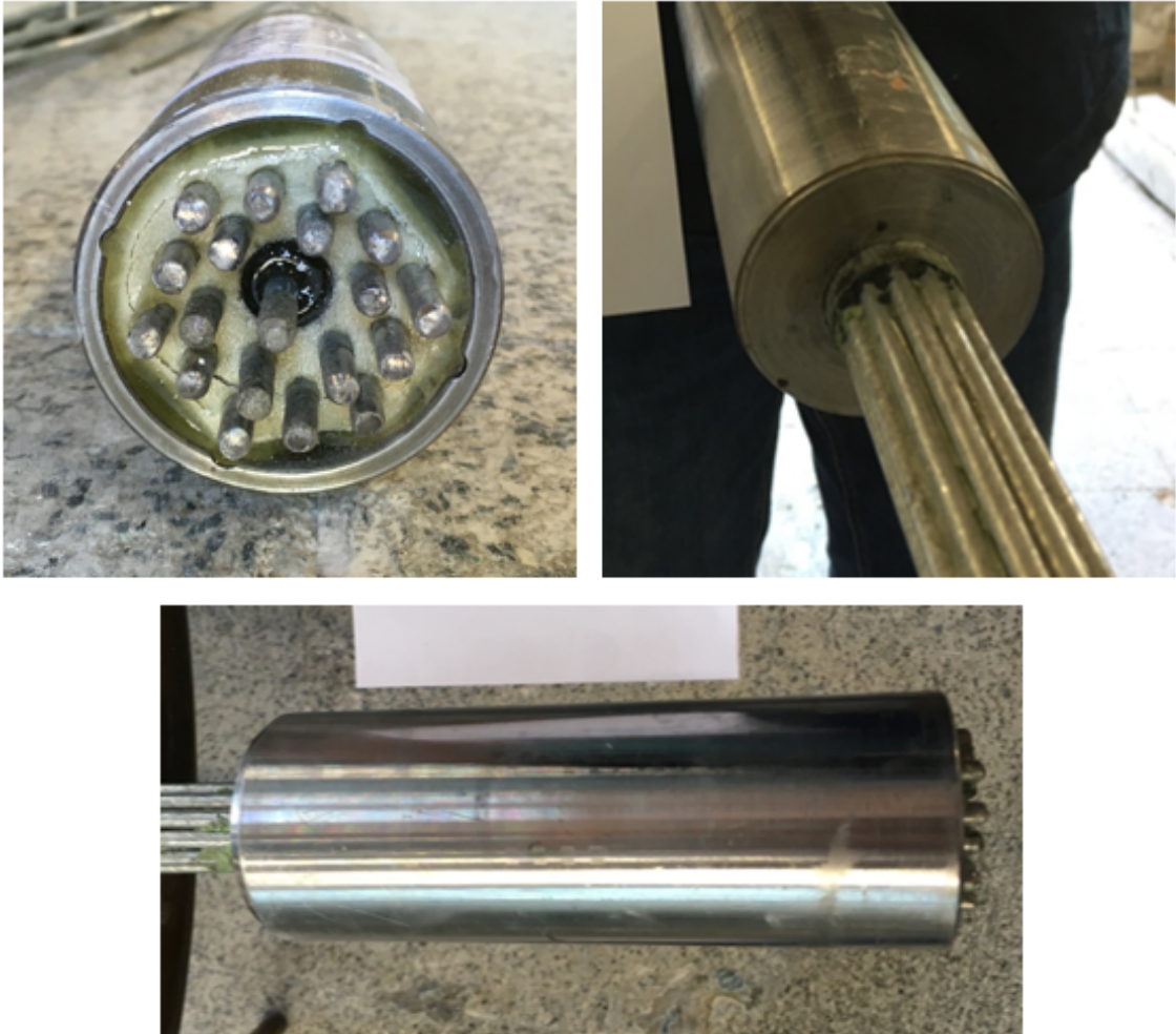
Figure 4.8. Condition of sockets after static test.
