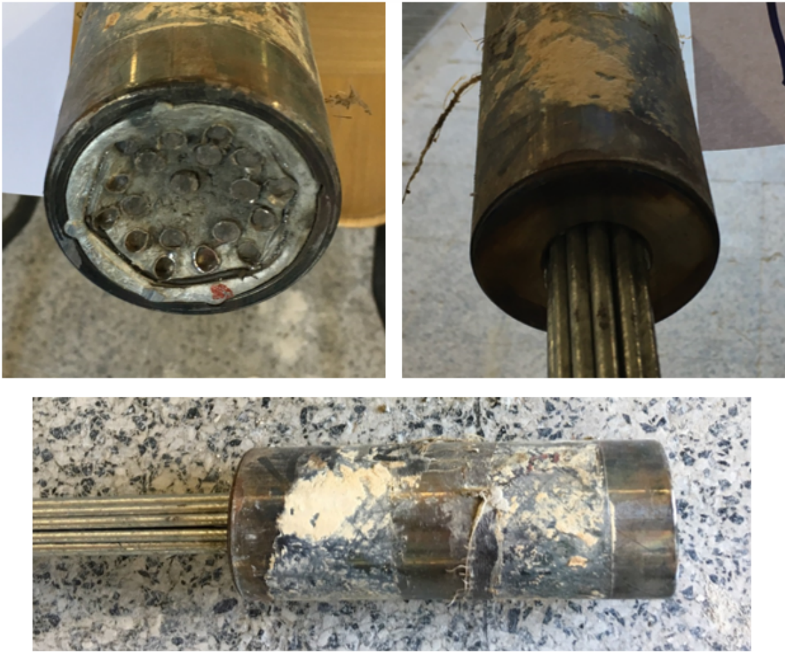
Figure 4.38. Condition of dead end socket after fire Test 5.
