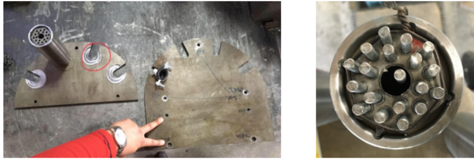
Figure 3.15. The socket holding plates (left-hand side) and the array plate and socket (right hand-side).
