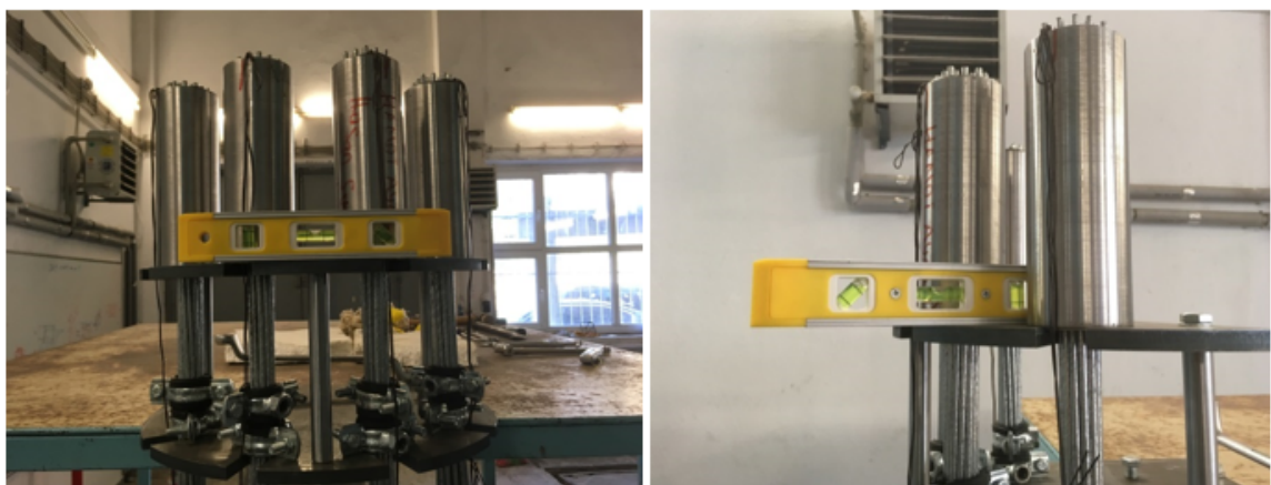
Figure 3.18. Adjusting and leveling the socket holding system.
