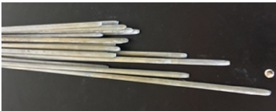
Figure 4.18. Discoloration of ruptured wires after fire Test 3.
