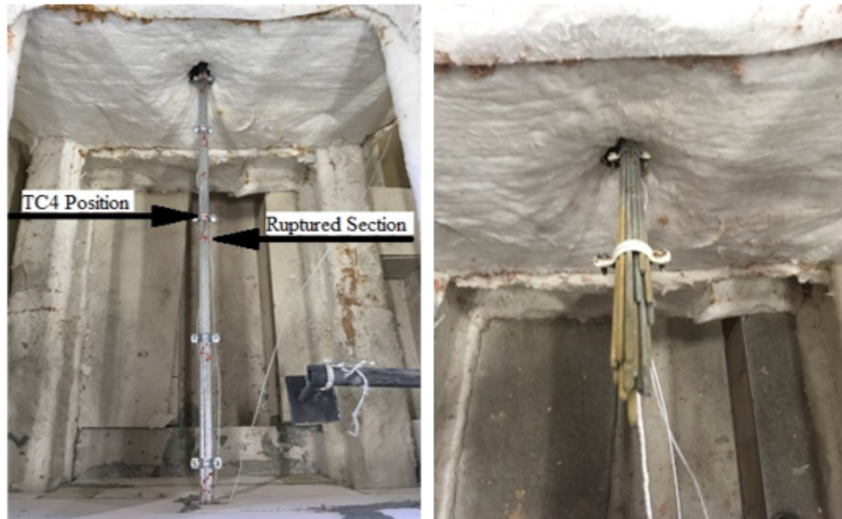
Figure 4.16. Ruptured section and TC4 position (left-hand side) and front view of rupture section (right-hand side).
