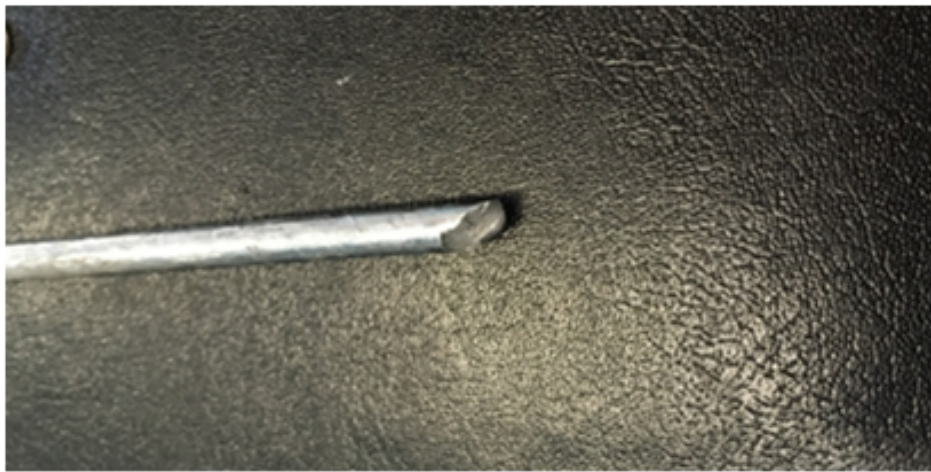
Figure 4.4. Typical shear wire fracture for S1.
