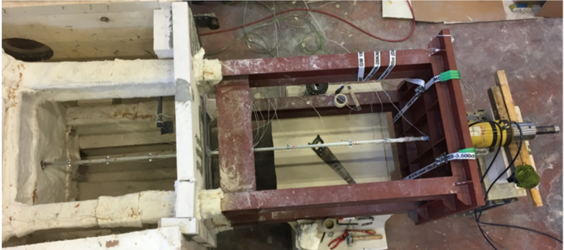
Figure 3.45. Top view of the cable setup for Fire Test.
