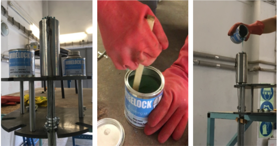
Figure 3.26. Preparing strand & socket, mixing, pouring.
