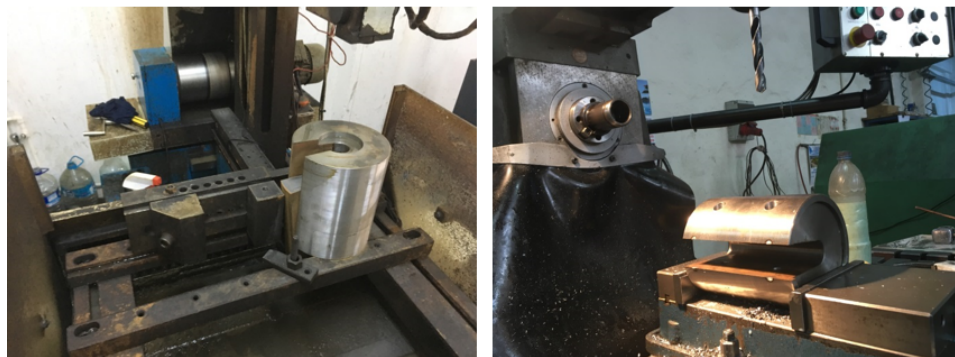
Figure 3.36. View of the socket locker after EDM cutting process (left-hand side) and the socket locker after threading (right-hand side).
