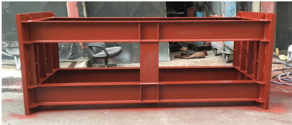
Figure 3.33. Side view of the steel test frame.
