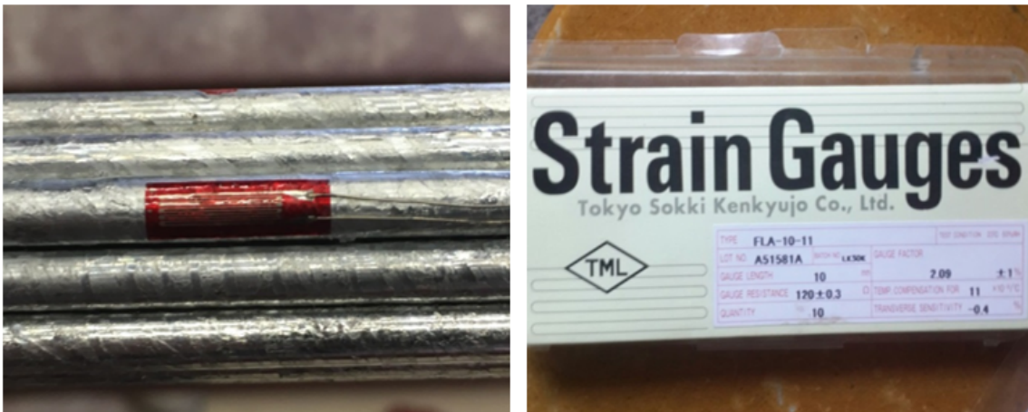
Figure 3.49. Strain gauge position on wire and TML strain gauge package.
