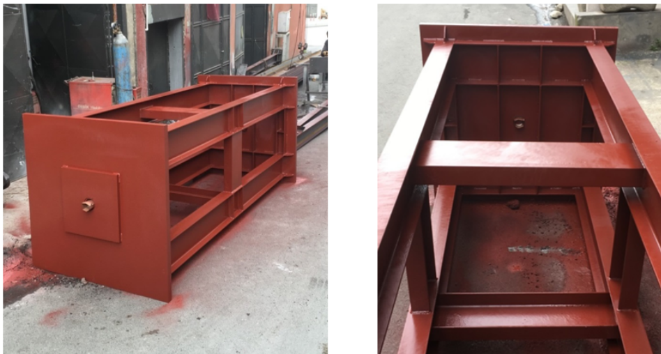
Figure 3.34. General views of the steel test frame.
