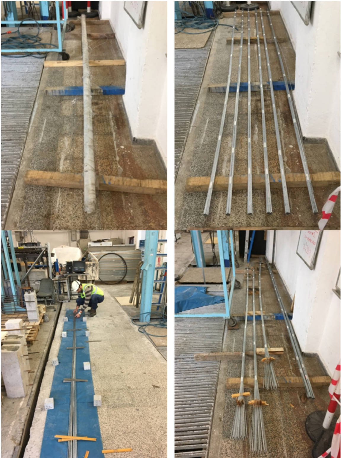
Figure 3.6. PWS specimens preparations for socketing.
