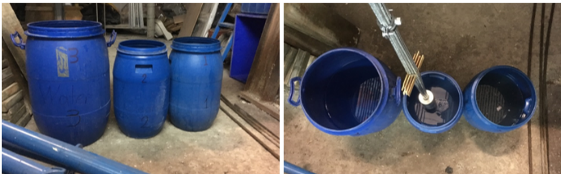
Figure 3.13. Caustic soda (#1), Flux cleaner (#2), Water (#3) and degreasing process for parallel wires.
