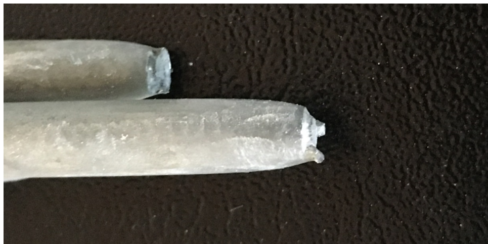
Figure 4.24. Typical cup and cone two wire break fracture for S4.
