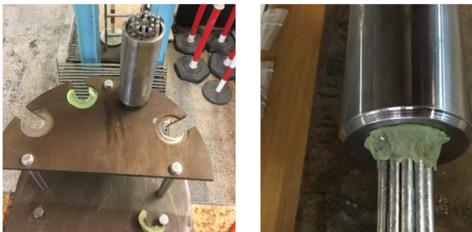
Figure 3.16. Top view of the specimen and socket holding system just before the socketing (left-hand side), sealing the base of the socket with clay for both socketing methods (right-hand side).
