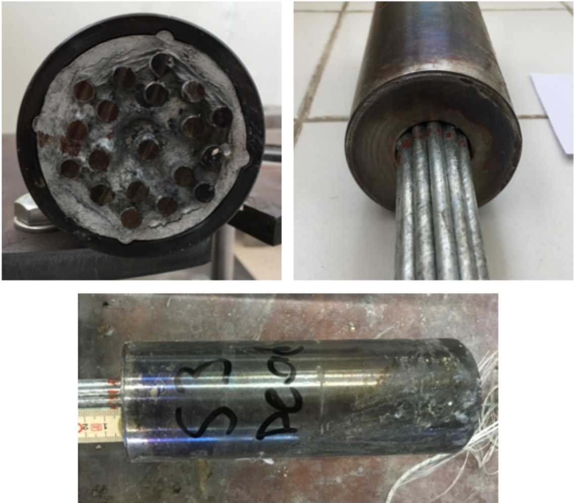
Figure 4.19. Condition of dead end socket after fire Test 3.
