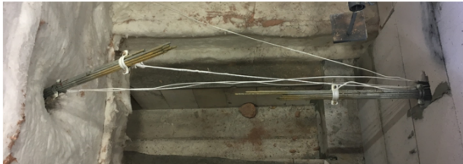
Figure 4.17. Failure view of S3 after fire Test 3.
