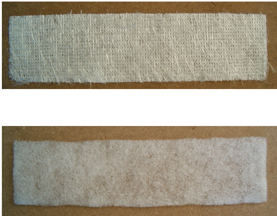
Figure 4.2 Fabric preform and core material used in the VARTM experiments.
