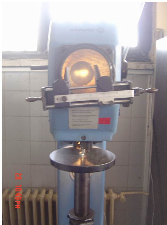
Figure 3.51. Magnified vision of the track formed by \text{Ø}2,5 mm. Wolfram Carbide ball
