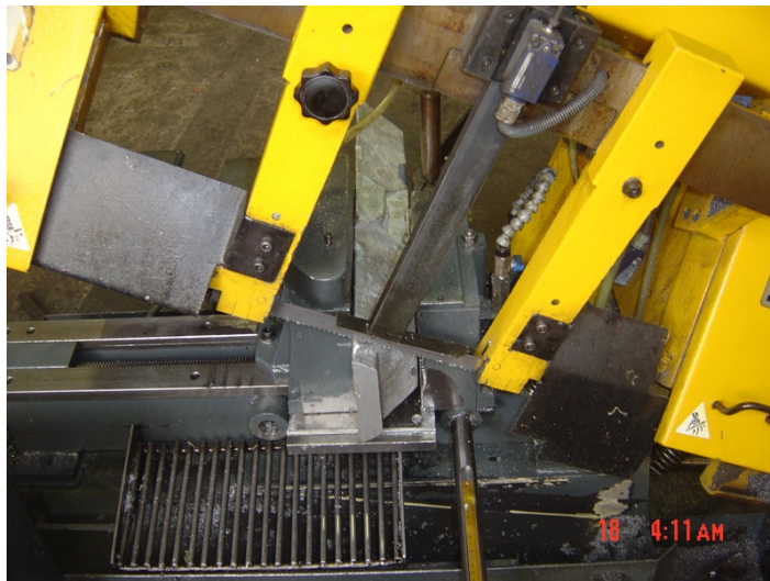
Figure 3.2. Cutting of ingots by Universal Horizontal Sawing Machine
