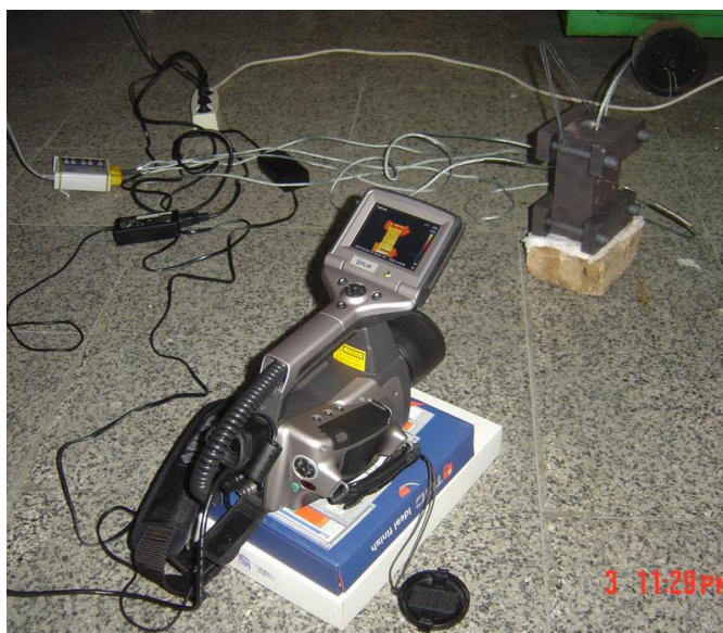
Figure 3.24. Recording of thermal distribution of die outer surface
