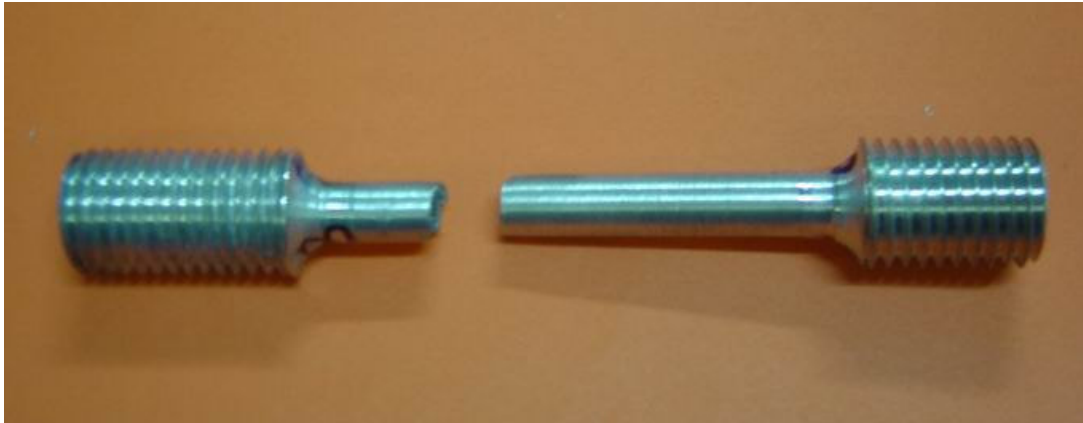
Figure 4.18. A broken specimen in tensile testing
