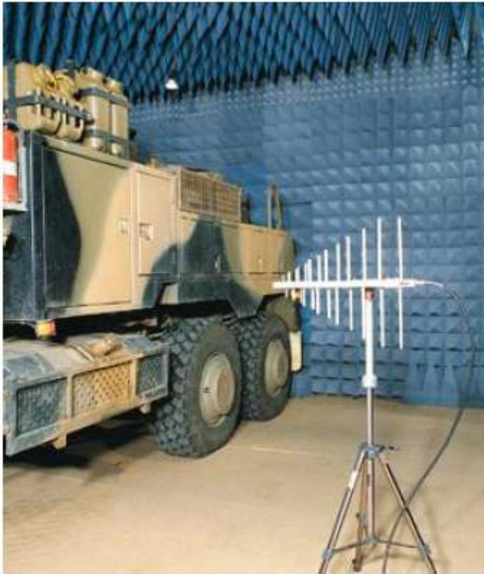
Figure 3.32 Full Anechoic Chamber
