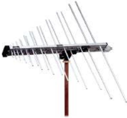
Figure 3.18 Log periodic dipole antenna
