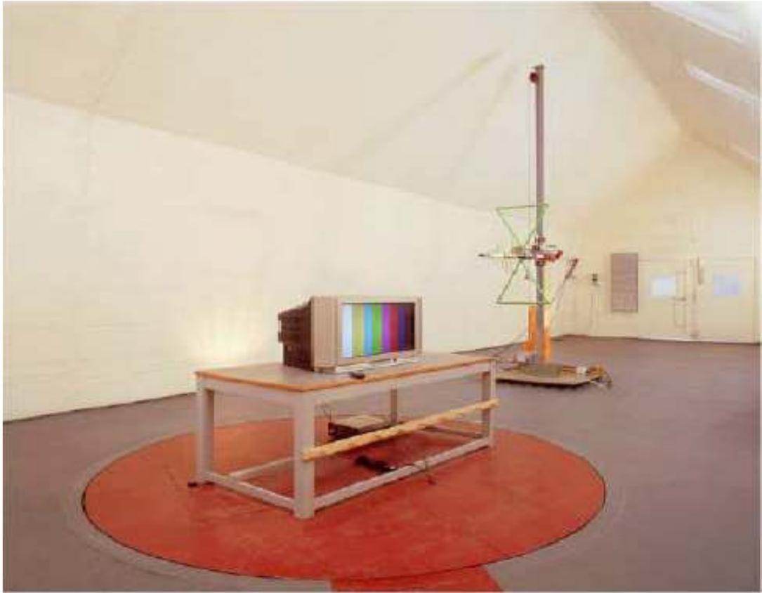
Figure 3.35 Covered Open Area Test Site
