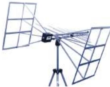
Figure 3.19 Bicon/log hybrid antenna
