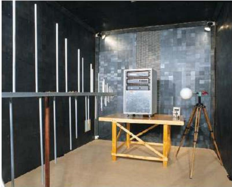
Figure 3.31 Semi Anechoic Chamber
