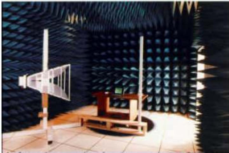
Figure 3.30 Typical anechoic chamber covered with ferrite
