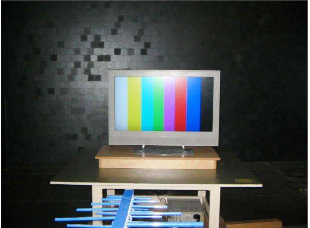
Figure 4.3 Measurement setup of a TFT LCD TV in Semi Anechoic Chamber
