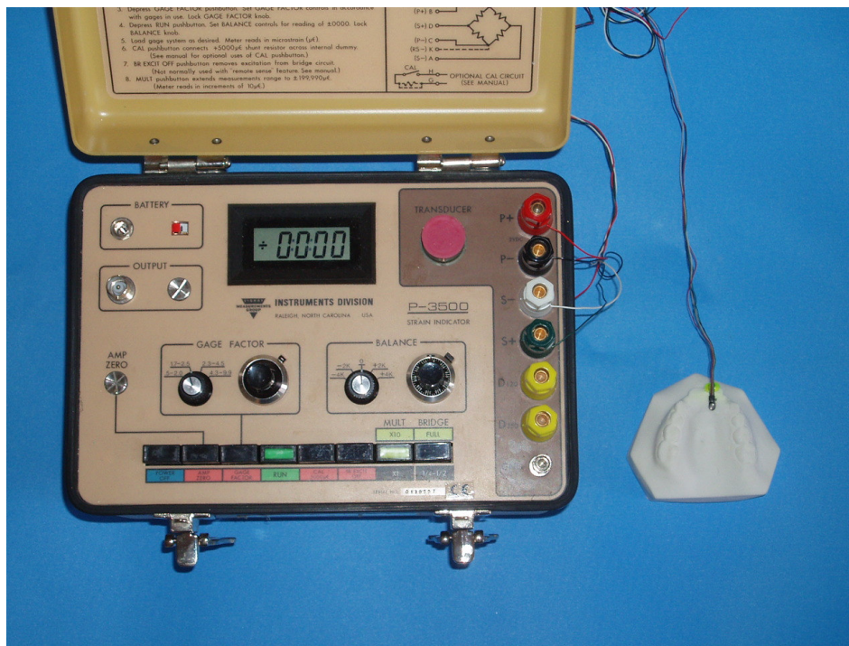
Figure 7. Full-bridge connection between strain indicator and pressure transducer
