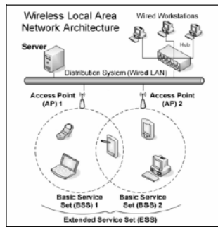
Figure1. A WLAN Architecture using BSS infrastructure
