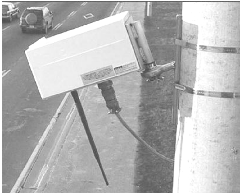
Figure 4.3. Side-fired RTMS ( www.rtms-by-eis.com )
