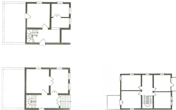
Figure 22, Plans of a traditional Buca dwelling and a dwelling with projection (Erpi, 1987, 250, 251)
