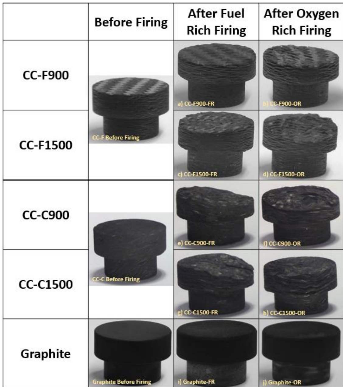
Figure 4.4 Appearance of Carbon Matrix Composites and Graphite Samples Before and After Tests: a) CC-F900-FR, b) CC-F900-OR, c) CC-F1500-FR, d) CC-F-1500-OR, e) CC-C900-FR, f) CC-C900-OR, g) CC-C1500-FR, h) CC-C1500-OR, i) Graphite-FR, j) Graphite-OR
