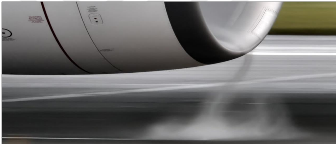
Figure 1.2. Example of Ground Vortices on Nacelle Body [5]
