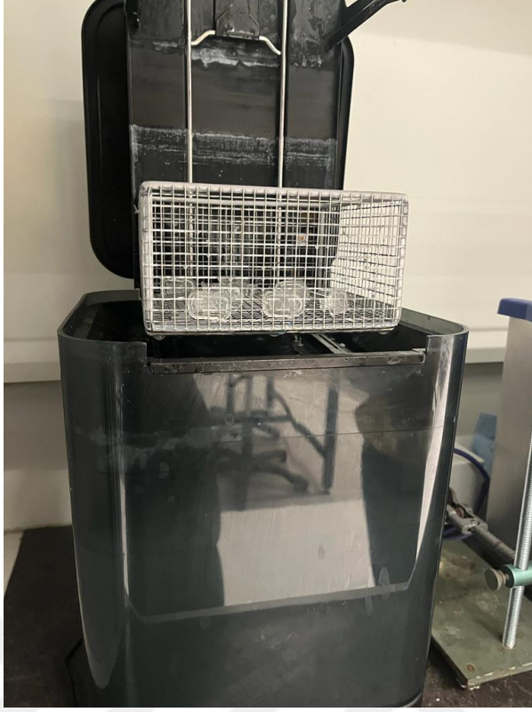
Resim 21: İzopropil alkol banyosu Form Wash (Formlabs®, Somerville, MA, ABD)
