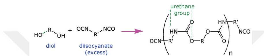
Figure 1. General reaction scheme for urethane formation[5].
