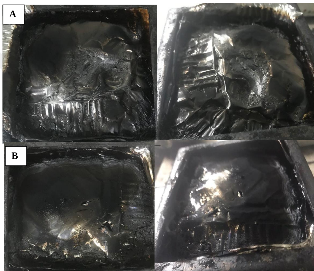
Figure 80. Images of residual chars from PU composites; A:5%MTB-MF 1:1-PU, B:5%MTB-MF 1:3-PU.
