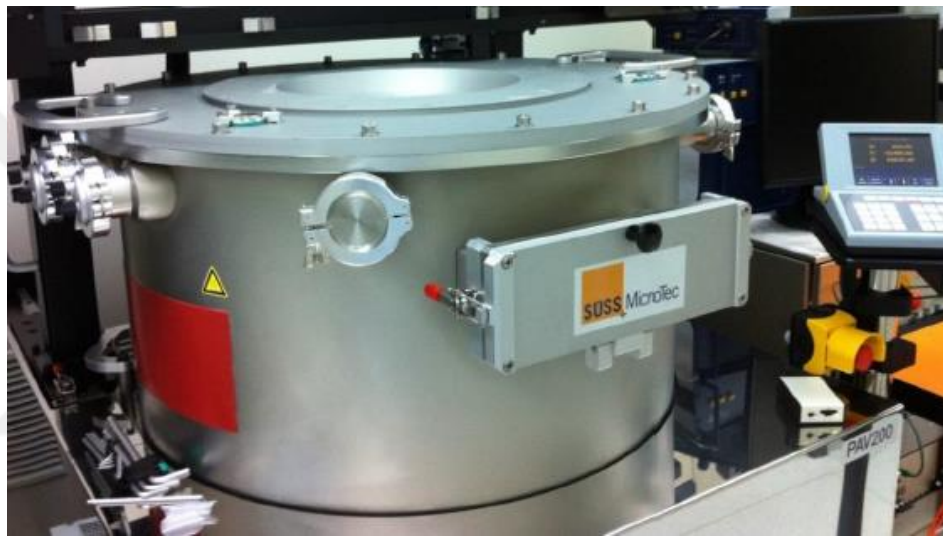
Figure 5.3: The resonance frequency test is performed by using the automatic probe station.
