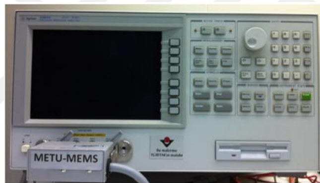
Figure 5.1: Agilent Precision Impedance Analyzer 4294A used during the C-V test.
