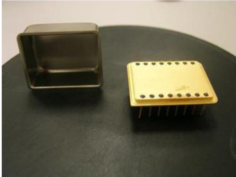
Figure 5.6: The 16 pin package used during the system level test.
