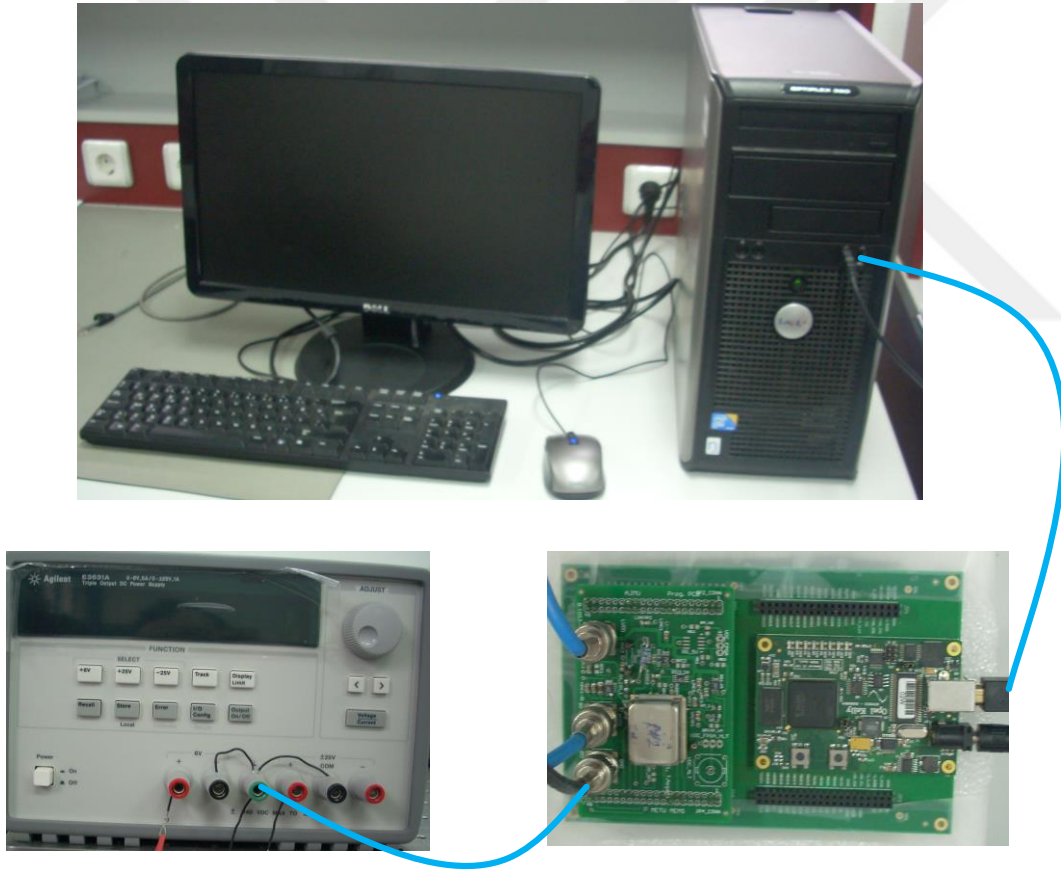
Figure 5.9: The test setup used during the system level test of the three-axis accelerometer.
