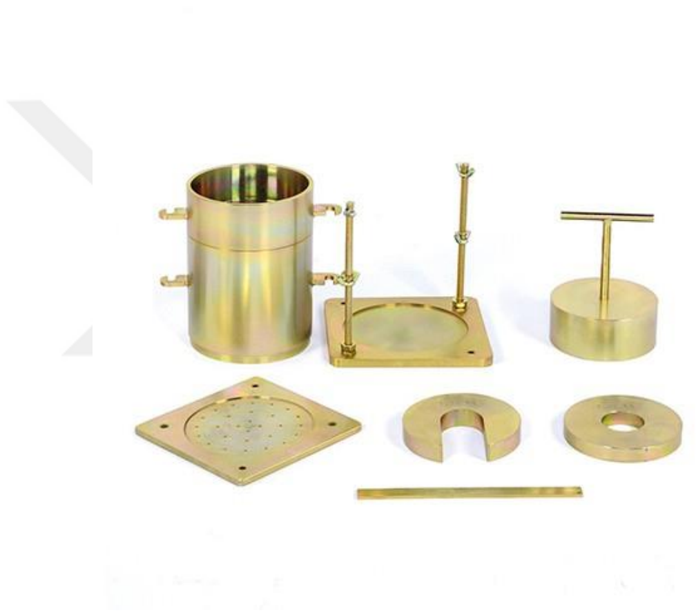
Figure 3.16. Compaction and sample preparation equipment for CBR test
