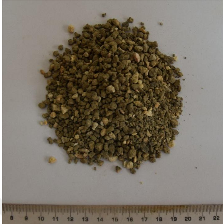
Figure 3.3. The reclaimed asphalt pavement (RAP) used during experiments
