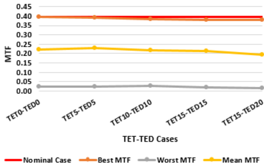
Figure 3.27 TET-TED cases with the image plane and the first group compensators. The analysis results indicate that if the optical and optomechanical components are made within these manufacturing tolerances, the goal means MTF value in the electro-optical system may be attained at a minimum of 20%.
