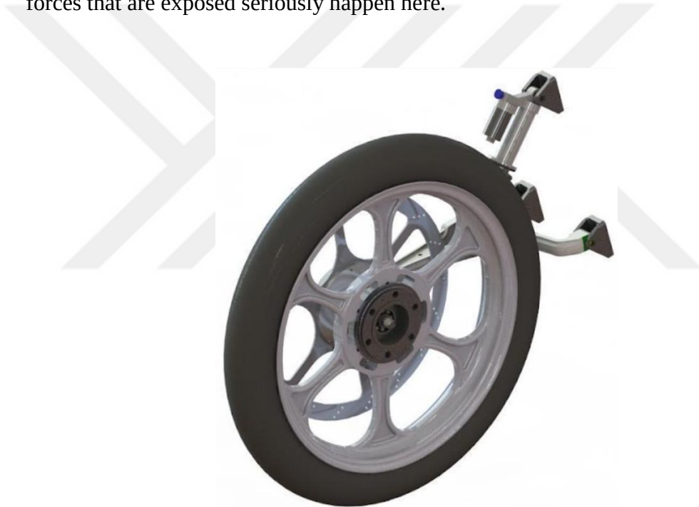
Figure 3.1 Rear suspension system of the Solaris 10 solar-powered EV
