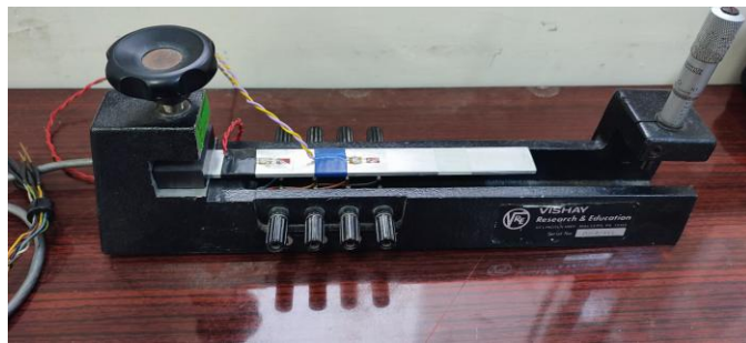
Figure 3.21 The cantilever flexure frame in which the experiment is performed (Personal archive, 2023)
