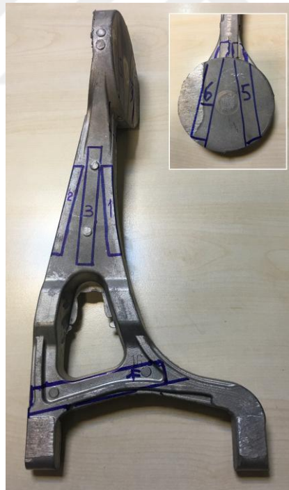
Figure 4.1 Tensile test specimens extracted from various regions of the rear swing arm (Personal archive, 2019)
