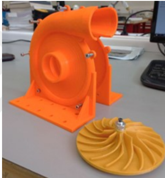
Figure 2.19: The printed volute and impeller before complete assembly
