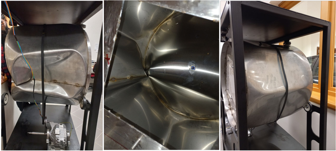
Figure 2.34: Buckled drum pictures.
