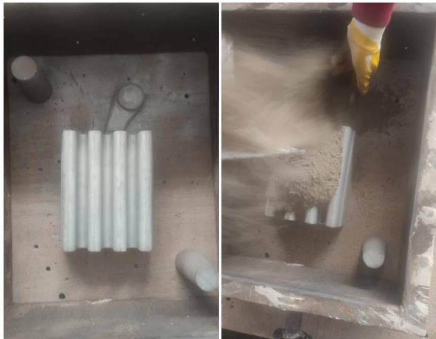
Figure 3.2: The molding process of tension chrod
