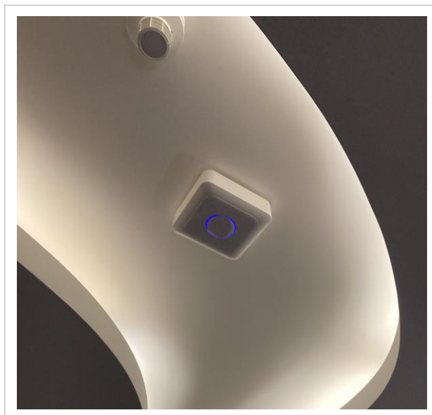
Figure C.2 The signal receiver used data from the tag with RFID technology.
