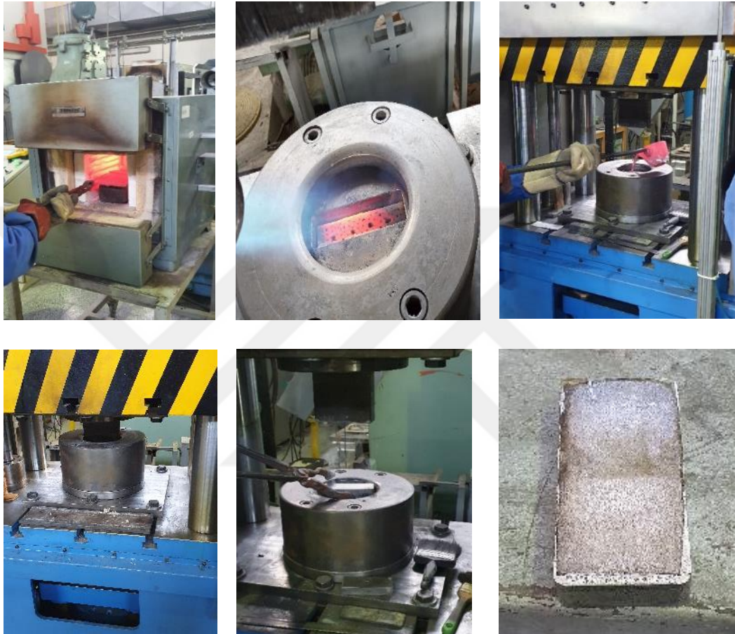
Figure 19. Experimental setup of squeeze casting and stages of MMC's processing and SiC infiltrated alloy composite.
