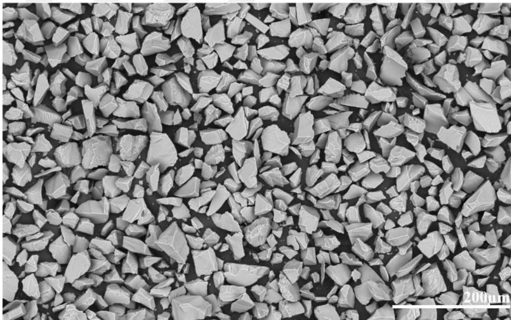
Figure 23. SEM image of raw SiC powder used for reinforcement.
