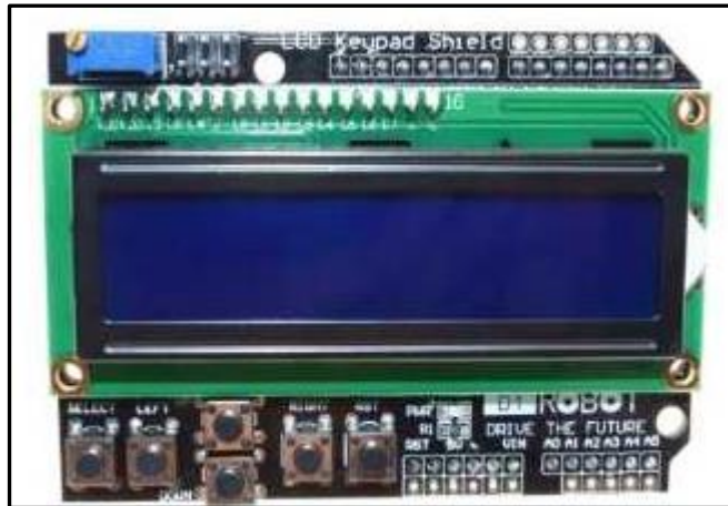
Figure 3.16 LCD keypad shield (14Core, 2013)
