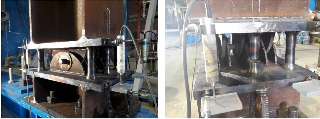
Figure 3.16: Permanent deformations and damages after PT2A Test
