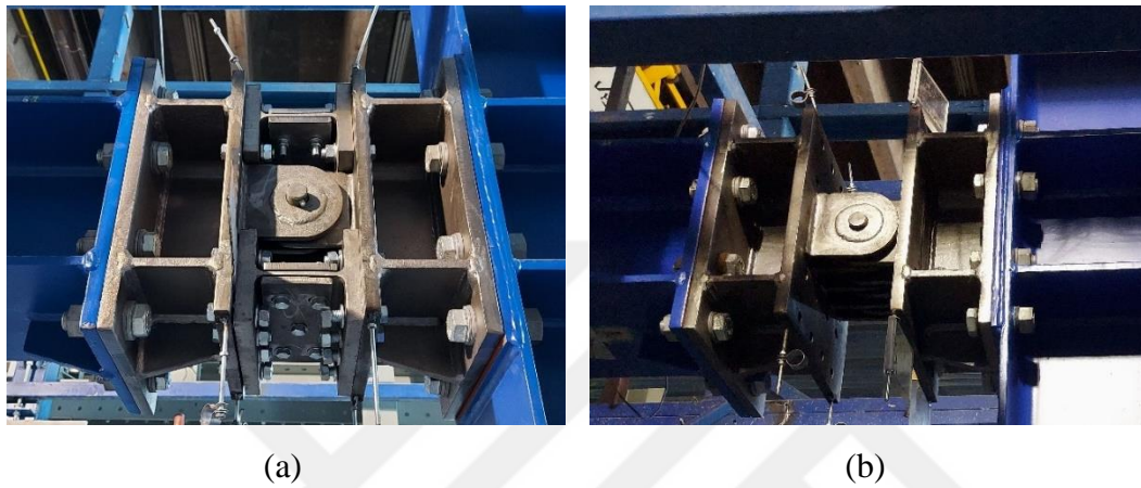
Figure 4.21: A P-Cell (a) with T/C components and (b) without T/C components, used as pin
