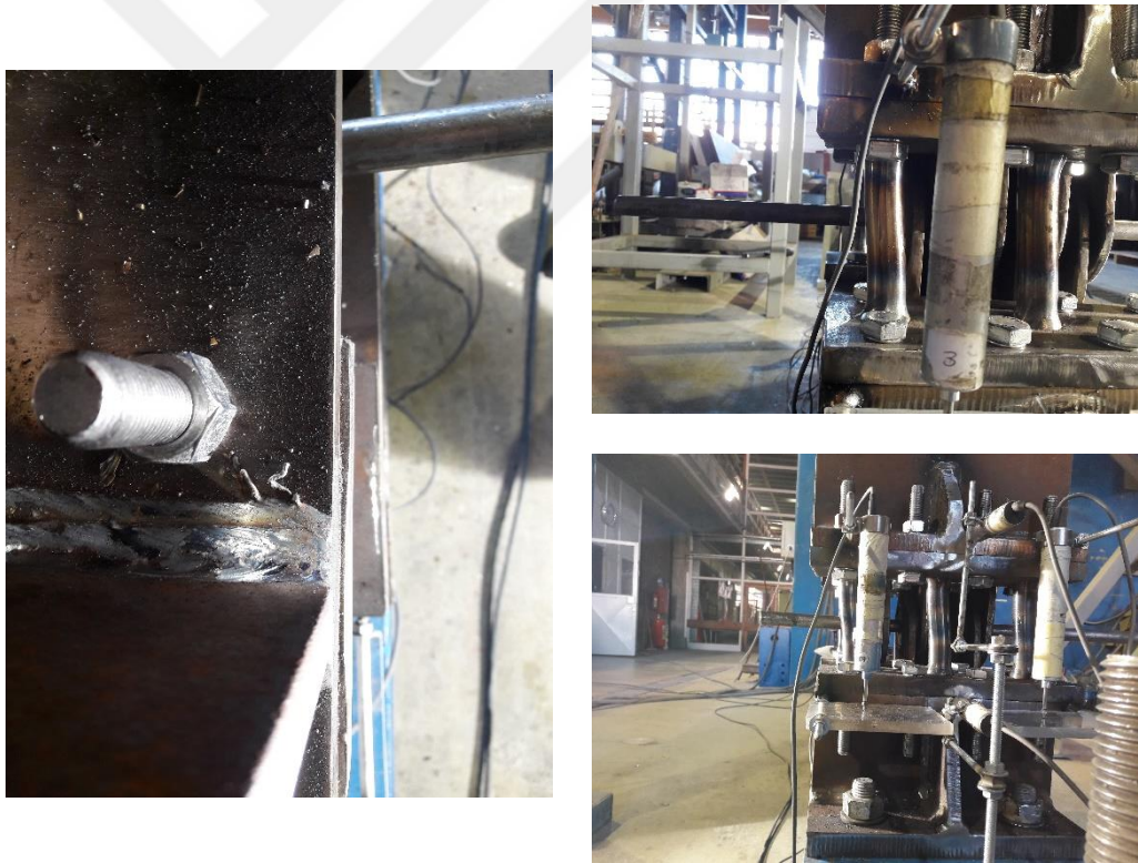
Figure 3.23: Observed torsional behavior on PT2B
