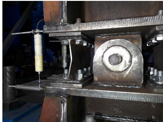
Figure 3.30: Permanent deformations and damages after PT3 Test
