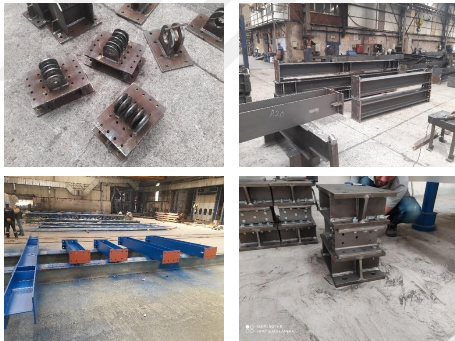
Figure 4.3: Production of P-Cells and frame members
