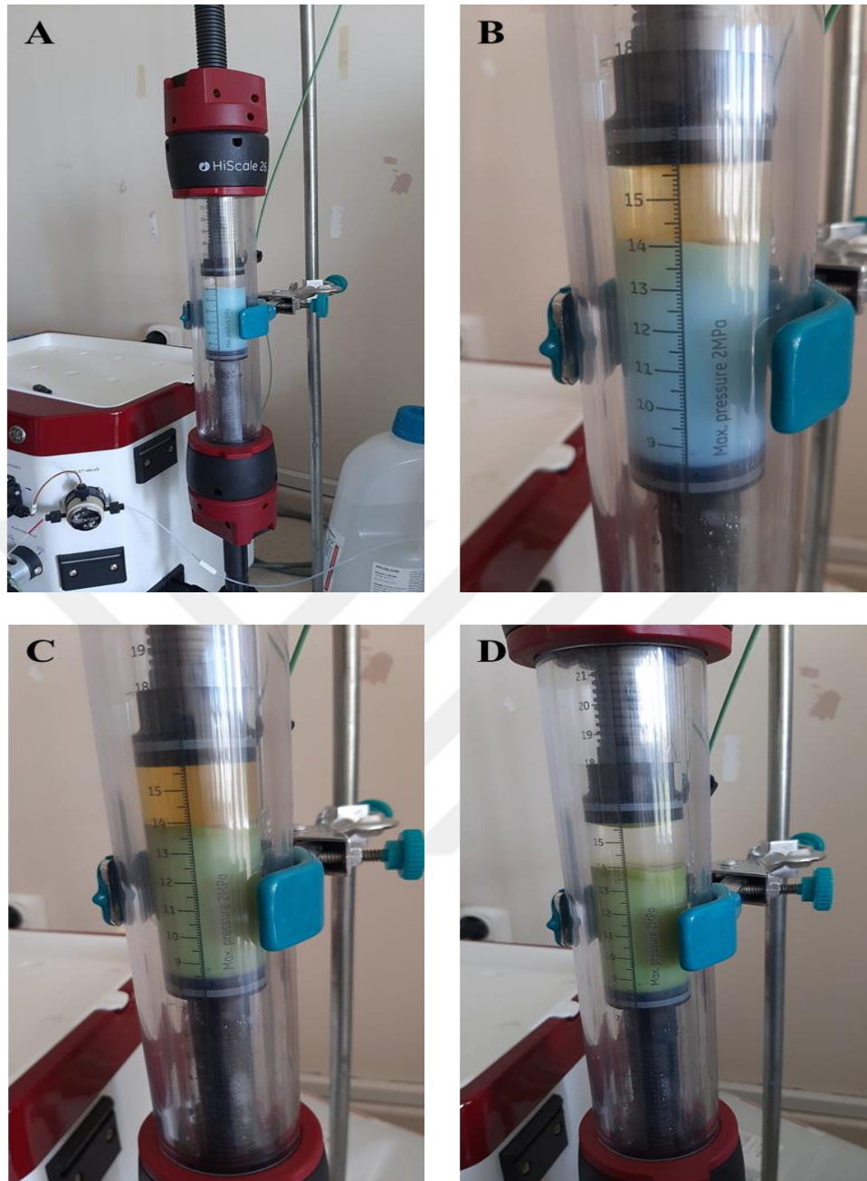
Figure 3.3. Ni column (HiScale™ 26/20) with Ni-NTA Resin (Ni Sepharose 6 Fast Flow) A) Conditioning of the column, B) First entry of the extracted material into the column, C) Transition of the extracted material during purification, D) Image of the column as a result of the purification process
