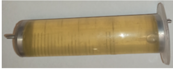
Figure 4.14: The conductivity measurements were performed using a cylindrical syringe. The resistance of the phantom was measured with the pins on the aluminum plates.
