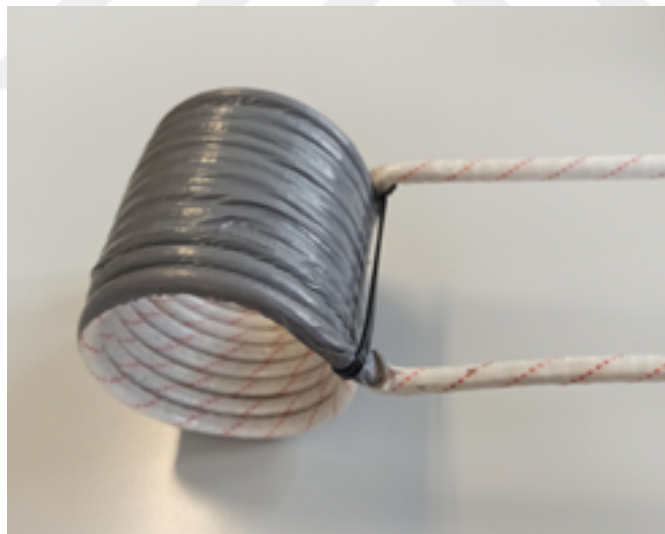
Figure 4.5: The geometry and dimensions of the constructed solenoid coil: 72 mm inner diameter, 82 mm outer diameter, 70 mm coil length, 5 mm pure copper wire diameter, and 6.3 mm copper wire diameter (including insulation band between windings).
