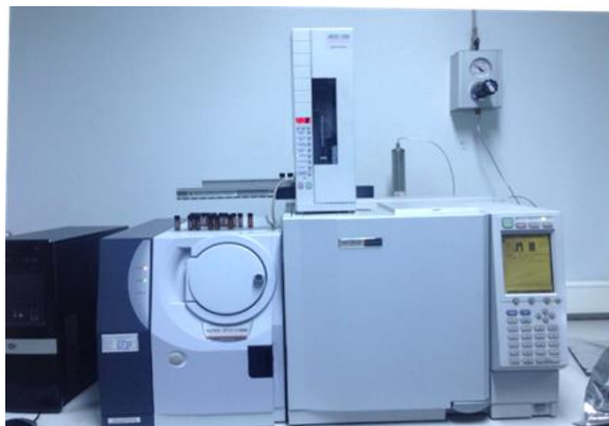
Figure 2.5. GC/MS used for pharmaceuticals in solution measurement.
