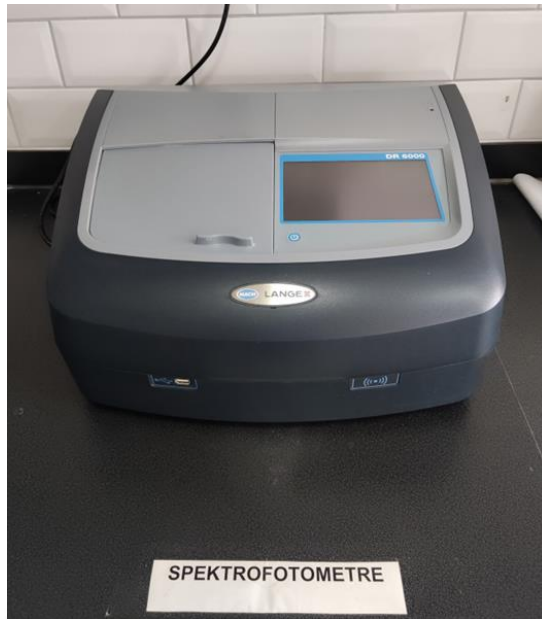
Figure 3.7 Spectrophotometer (HACH LANGE DR 6000).
