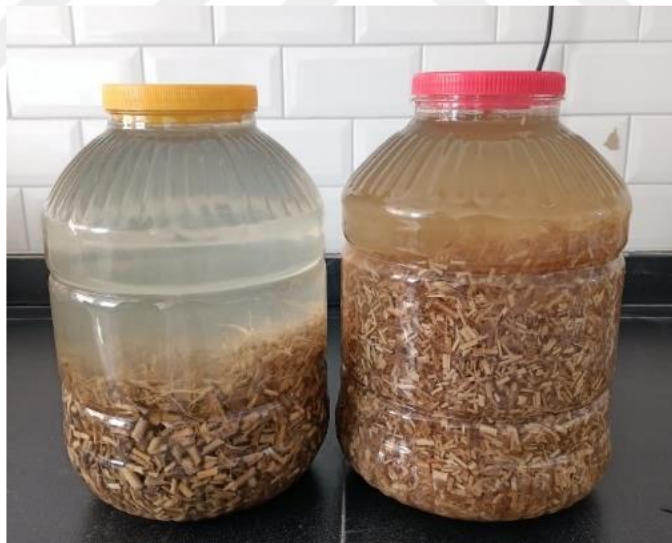
Figure 3.1 Chopped hemp submerged in water for its saturation.
