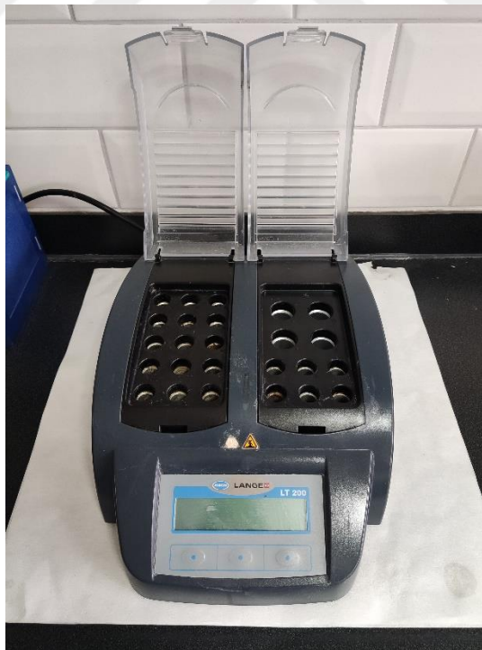
Figure 3.6 Thermarator Device (Hach Lange LT200).
