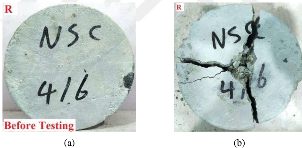
Figure 4.16. Reference unheated NC disk specimens (a) before testing (b) after testing.
