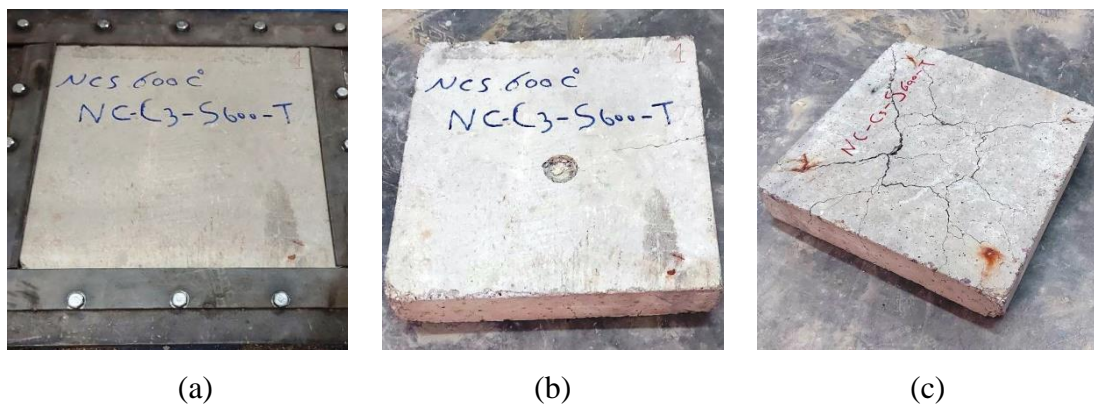
Figure 5.42. Pictures of NC four-ends restricted plate heated to 600 °C (a) before testing (b) top surface after testing (c) bottom surface after testing.
