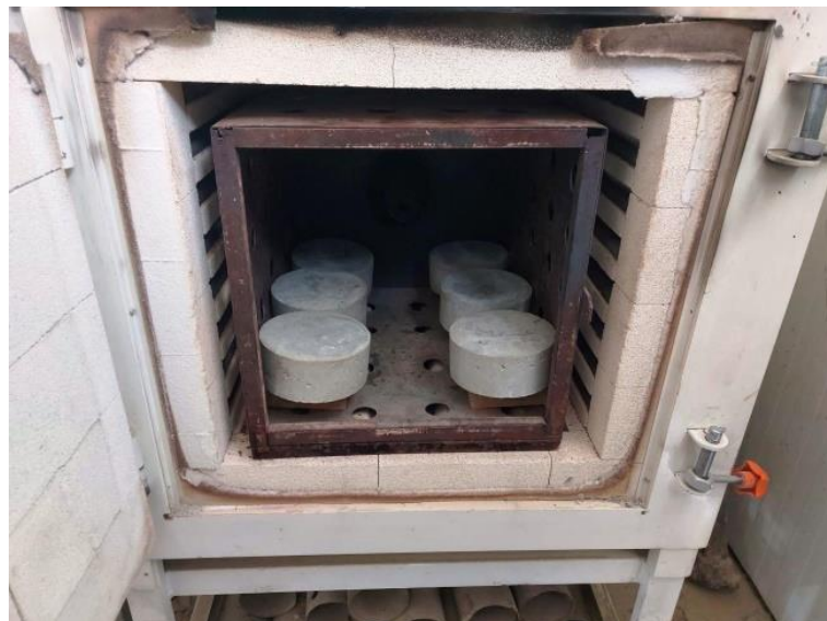
Figure 3.29. Placement of test specimens inside the furnace.
