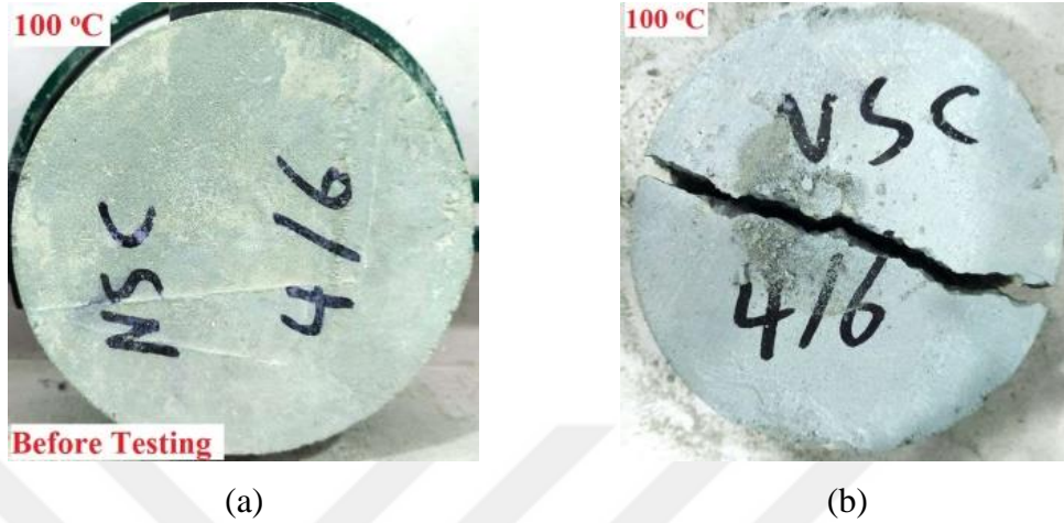
Figure 4.17. NC disk specimens subjected to 100 °C (a) before testing (b) after testing.
