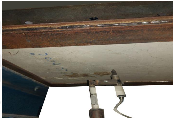
Figure 3.16. LVDT is placed under the center of the specimen.
