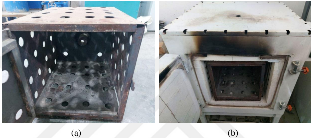
Figure 3.28. Protection of the electrical furnace using a steel cage (a) the steel box-cage (b) the final internal view of the furnace.
