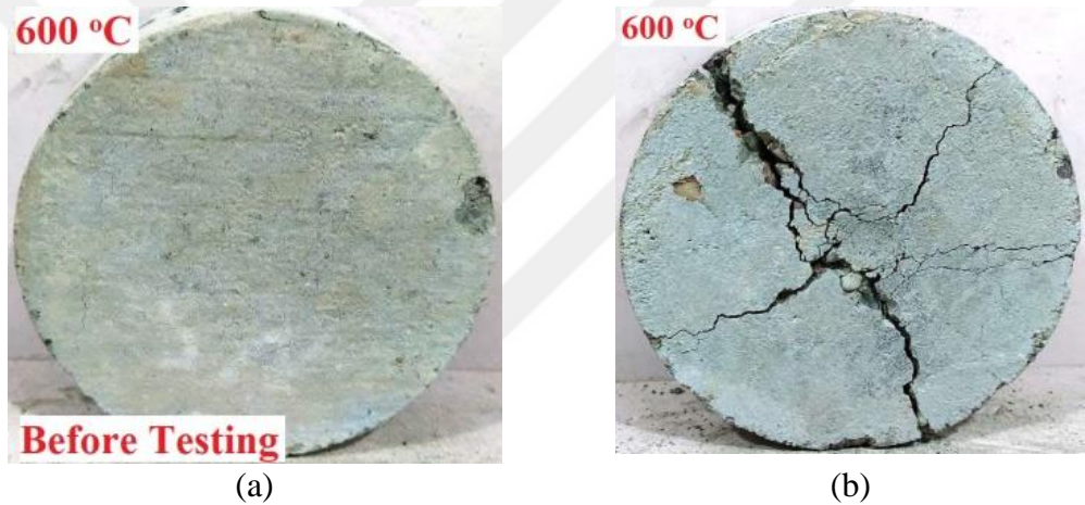
Figure 4.22. NC disk specimens subjected to 600 °C (a) before testing (b) after testing.
