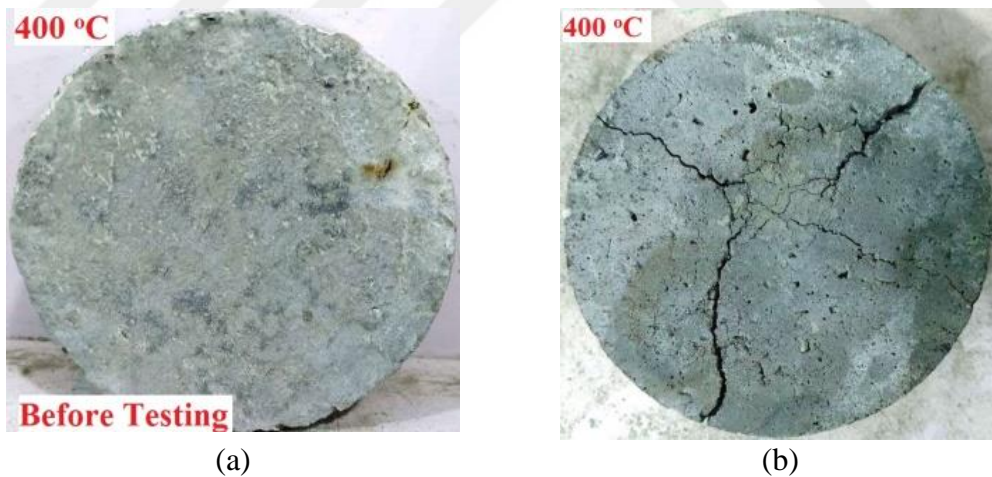
Figure 4.20. NC disk specimens subjected to 400 °C (a) before testing (b) after testing.
