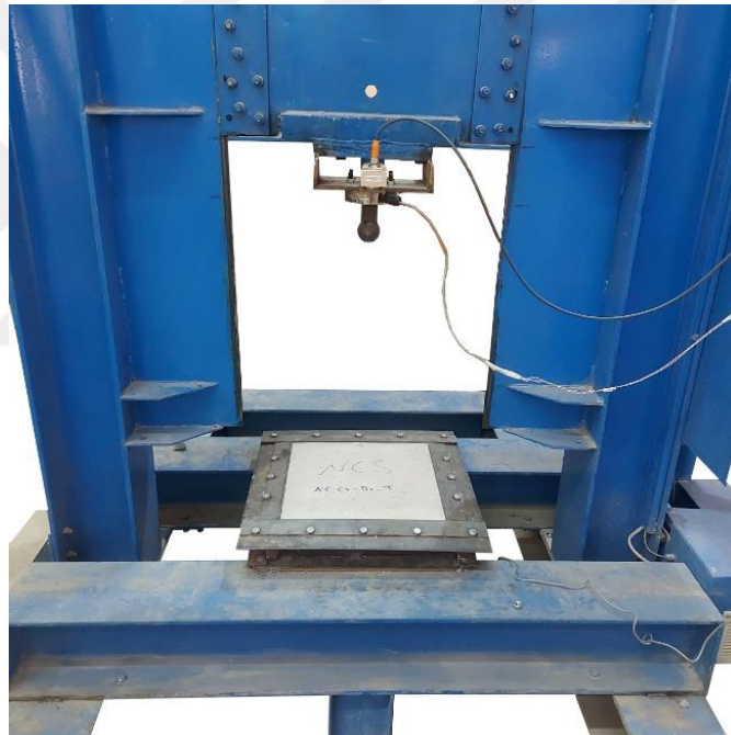
Figure 3.14. The load cell was attached to the impact point that falls.
