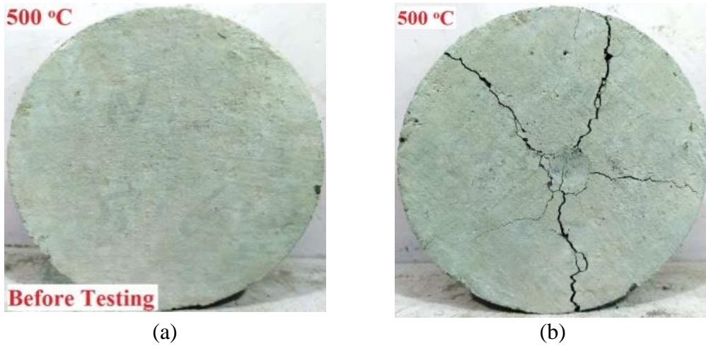
Figure 4.21. NC disk specimens subjected to 500 °C (a) before testing (b) after testing.
