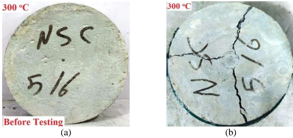
Figure 4.19 NC disk specimens subjected to 300 °C (a) before testing (b) after testing.
