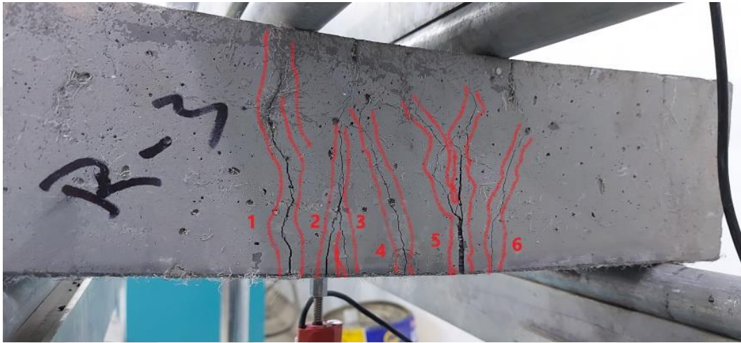
Figure 4.7. multi-cracking failure of tested prisms.
