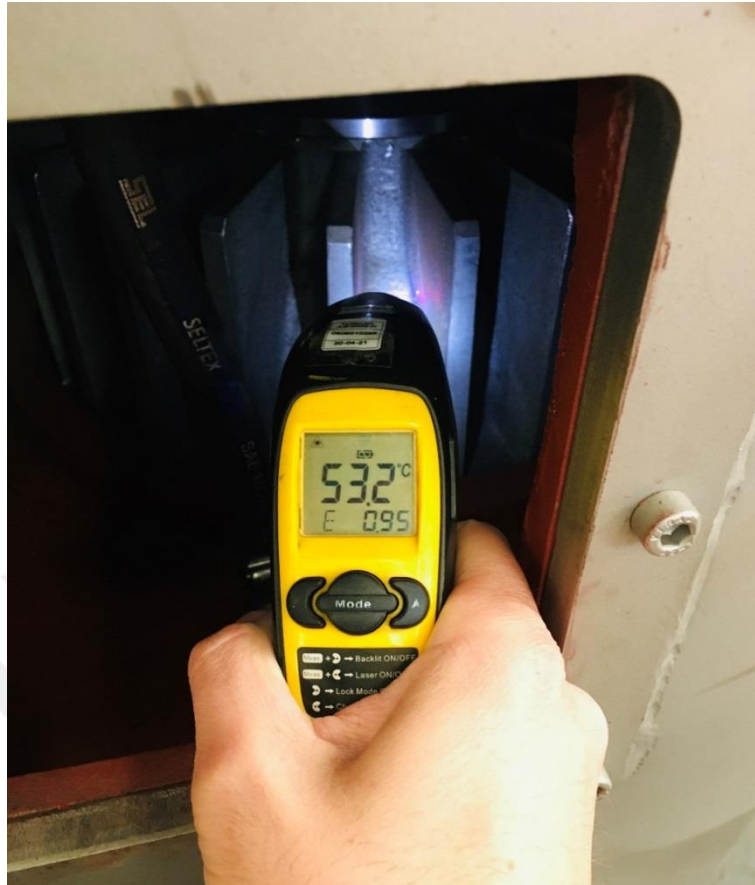
Figure 4.5. With fin oil chamber temperature at last sample.
