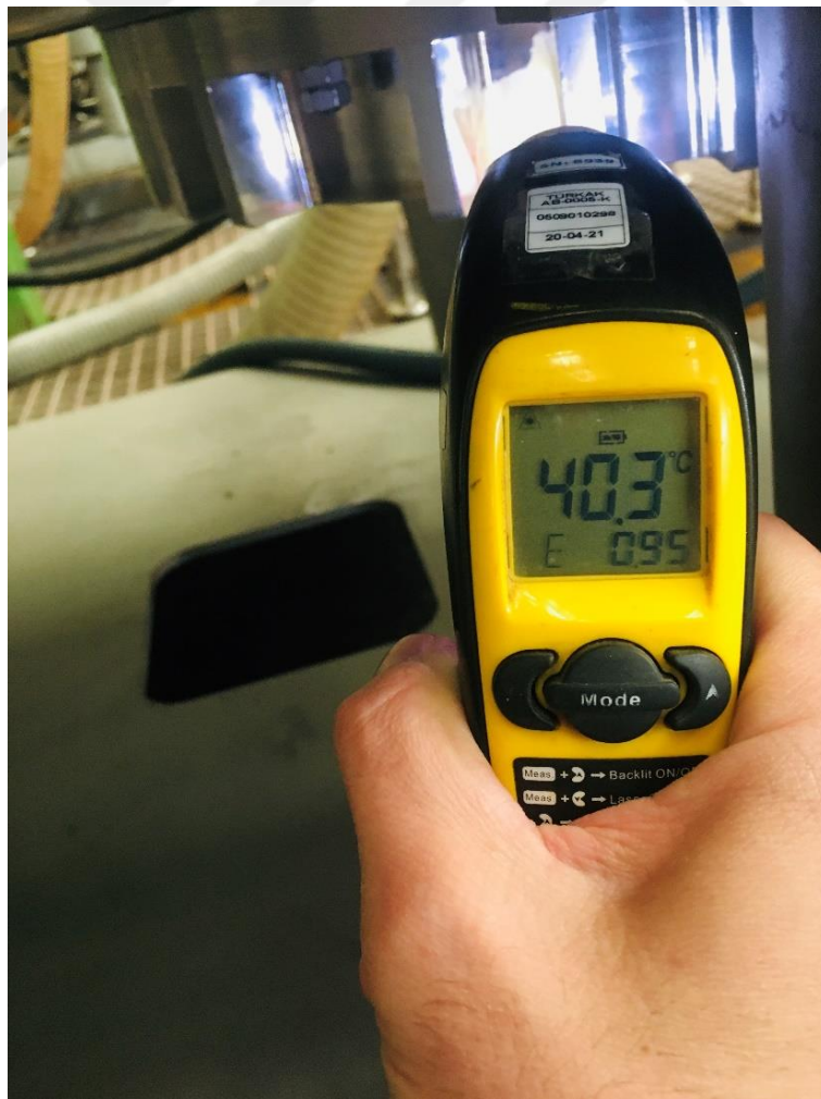
Figure 4.2. First temperature without fins part before machine start.
