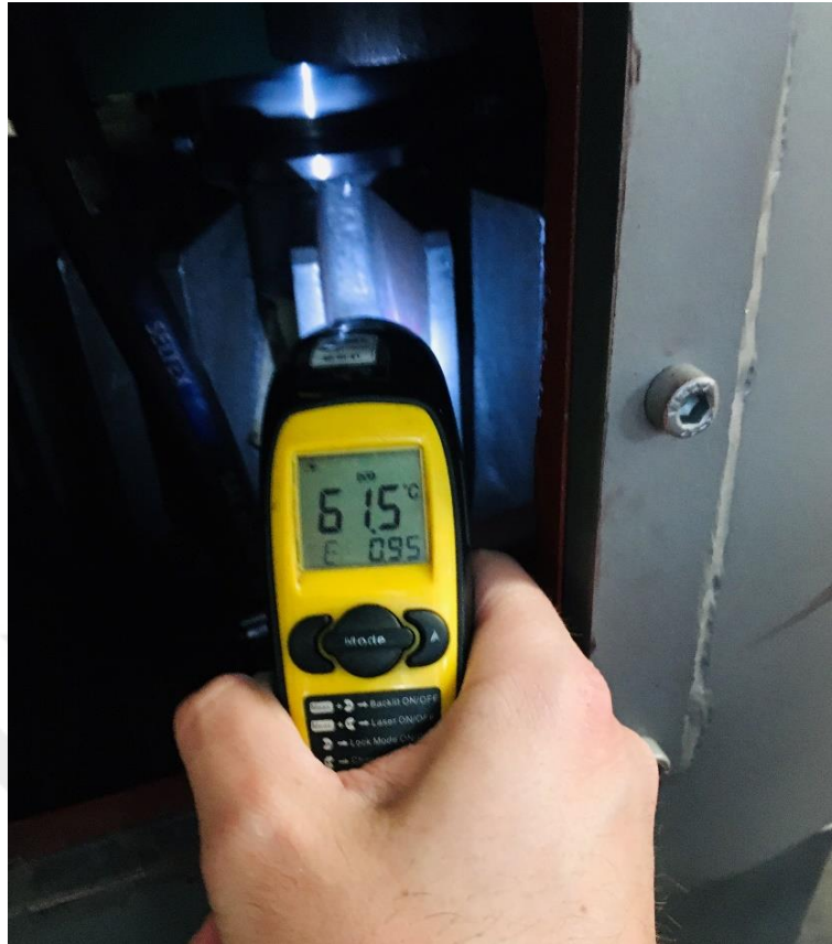
Figure 4.3. Without fin oil chamber temperature at last sample.
