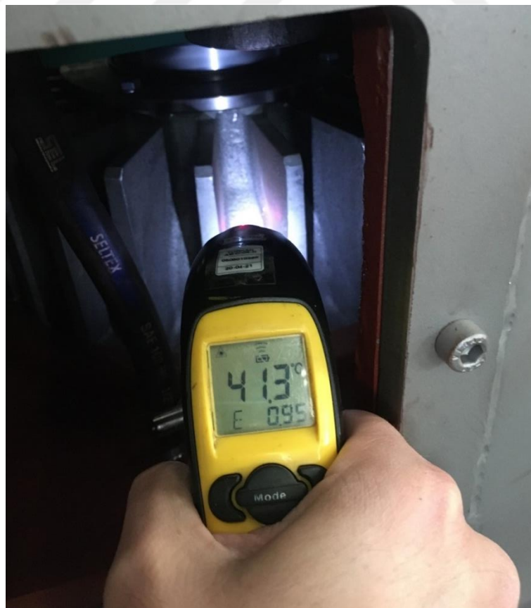
Figure 4.4. First temperature part with extended fin oil chamber before machine start.
