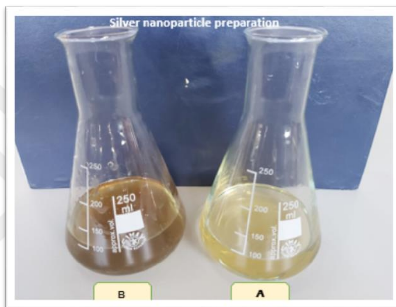
Figure 4.8 Preparation of the silver nanoparticles (A) silver nitrate solution (B) formed silver nanoparticles
