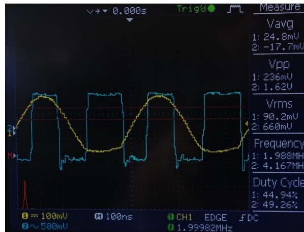
Figure 5.4-1 LVDS's input (channel 2) and output (channel 1)
