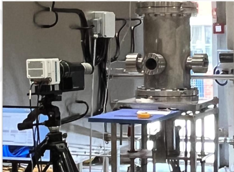
Figure 3.6. The chemiluminescence measurement system
