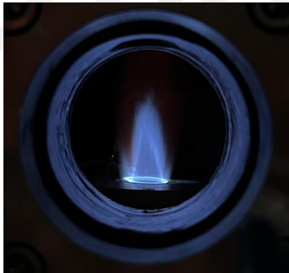
Figure 3.5. The turbulent premixed flame with 0.8 equivalence ratio with no hydrogen addition
