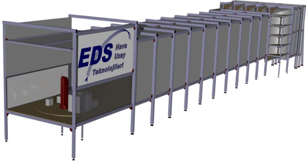
Figure 1.8 : EDS atmospheric boundary layer wind tunnel.
