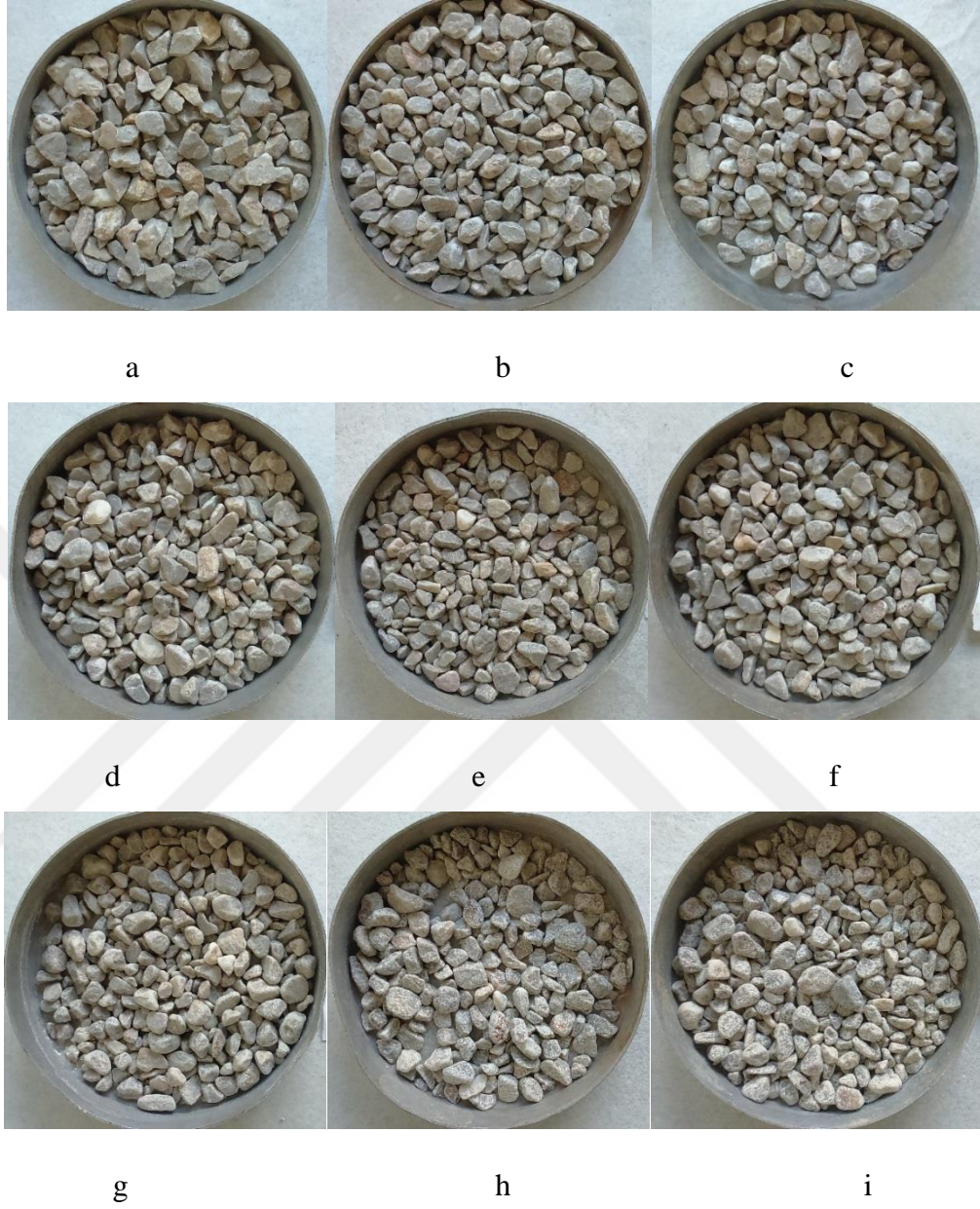
Şekil 3.7. (a) 0 tur, (b) 5000 tur, (c) 10000 tur, (d) 15000 tur, (e) 20000 tur, (f) 25000 tur, (g) 30000 tur, (h) 50000 tur ve (i) 100000 tur
