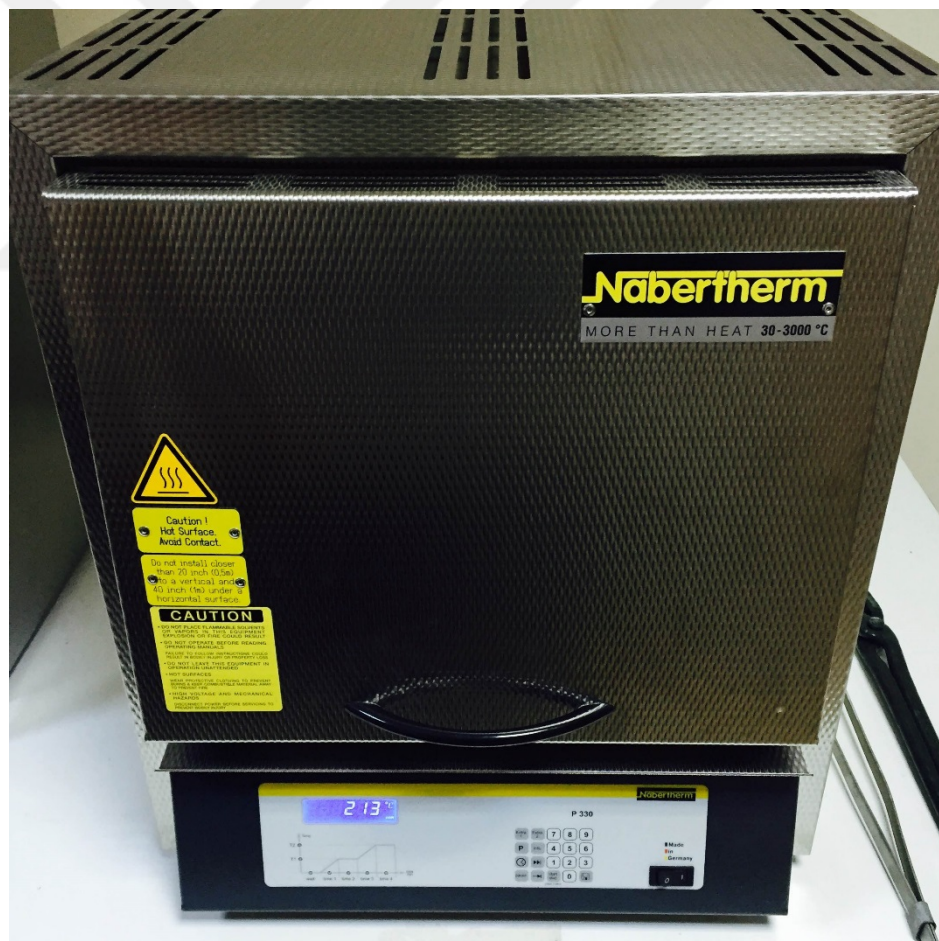
Figure 3.1 The furnace used in the experiments (Nabatherm model P330)
