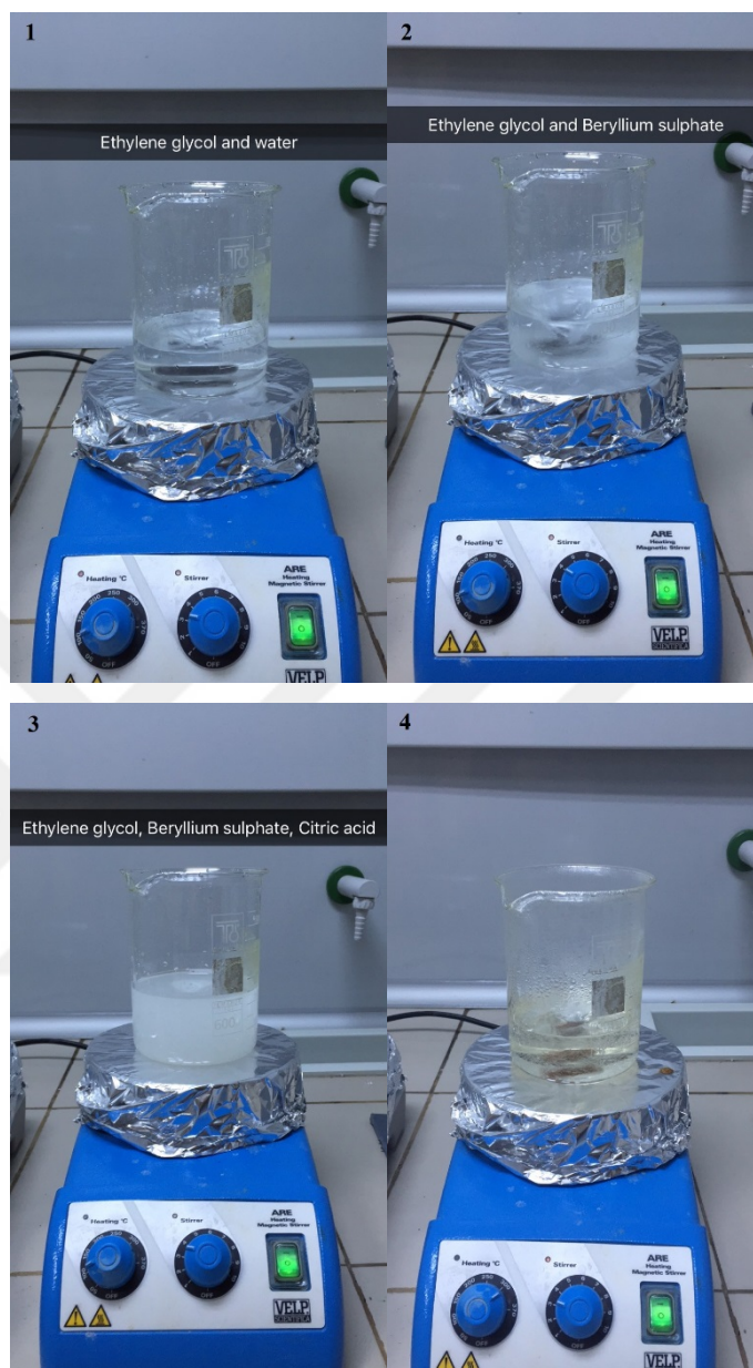
Figure 4.1 The first step of BeO synthesis, (1) the solution of ethylene glycol and water, (2) beryllium sulphate in ethylene glycol, (3) added citric acid to solution, (4) after dissolving all the ingredients
